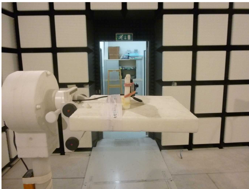
Photo 2: EUT at the anechoic chamber
