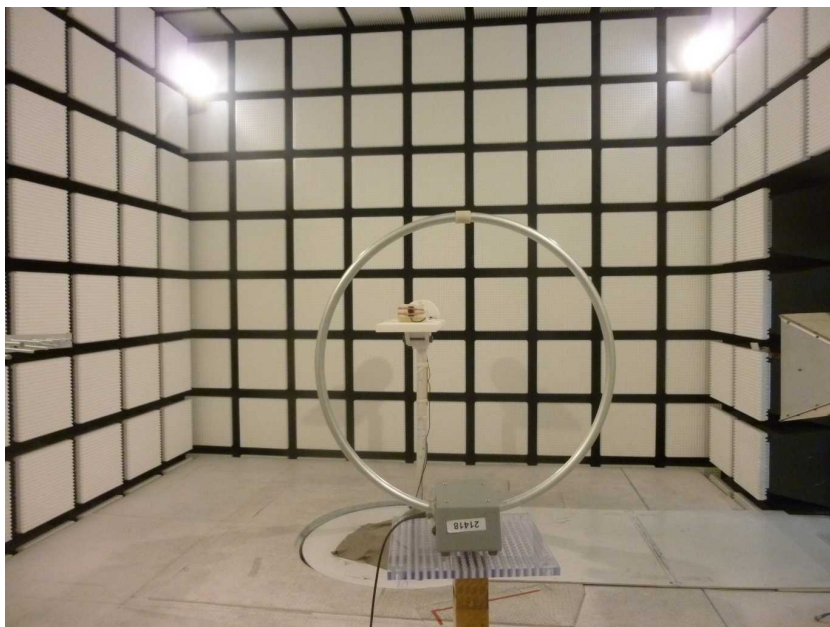
Photo 6: EUT at the anechoic chamber
