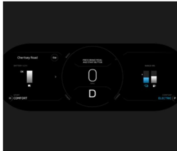
3. The ignition will switch on, the oil temperature, water temperature and fuel gauges will operate and several of the warning lights will illuminate as a self-test. The Driver Display will fully illuminate.
