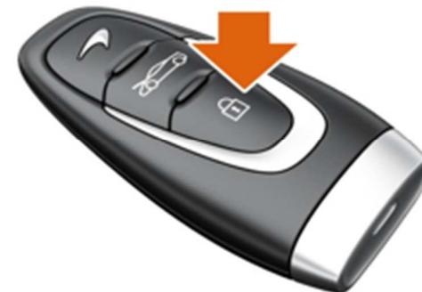
In the event of continuous anti-trap events, press the lock button for a few seconds. The window will continue to raise until you remove your finger from the lock button. Only attempt this if the above methods do not resolve the problem.
