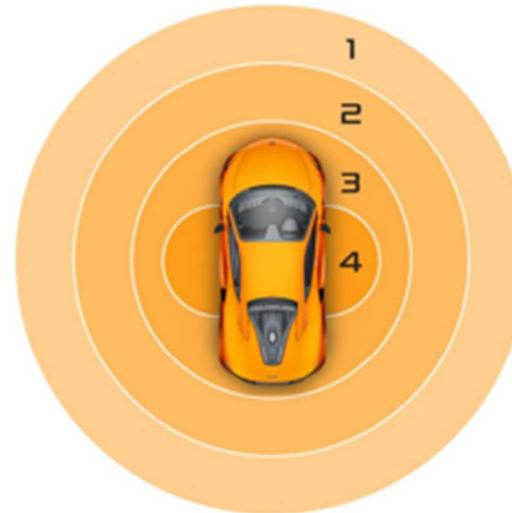
Sensors detect the location of the key fob around the vehicle, in the following zones:
