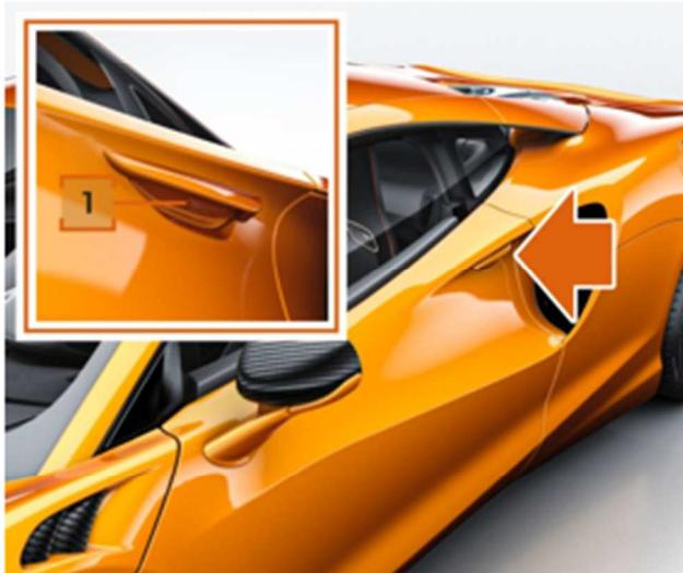
1. Press the handle (1) firmly to unlatch the door.
