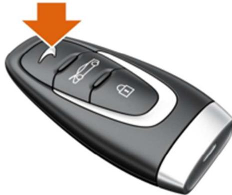
To unlock the vehicle, using the key fob, press the unlock button. The front, rear and side direction indicators (market specific) flash twice and the anti-theft alarm system will be deactivated.
