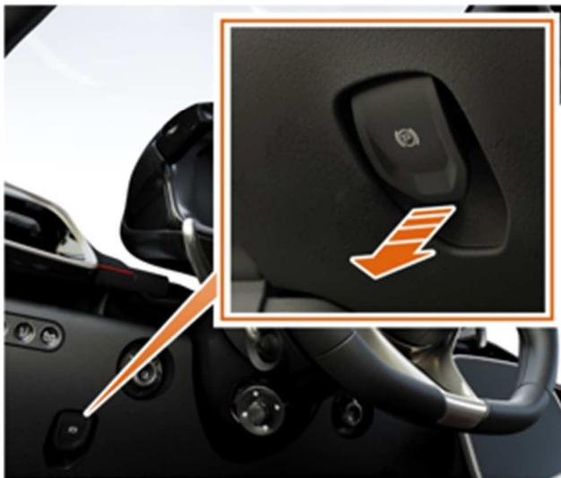
To engage the parking brake, pull the switch outwards, the red parking brake applied status light on the Driver Display illuminates.
