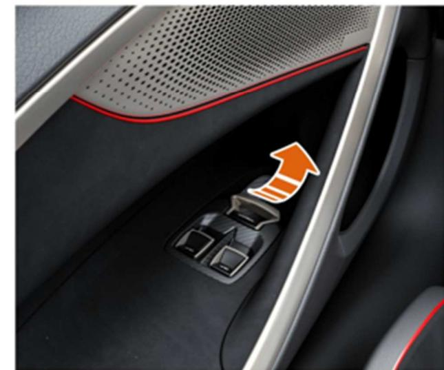
Pull door handle upwards, in direction of arrow, and push the door outwards until the opening mechanism takes over. The door will then swing outwards and upwards automatically.
