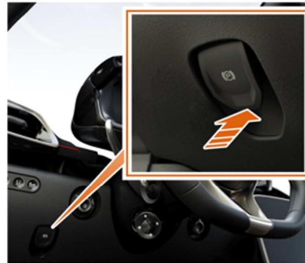
To disengage the parking brake, keep the brake pedal depressed and push the parking brake switch inwards, the red parking brake applied status light on the Driver Display extinguishes.
