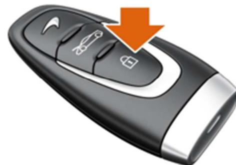
If either of the doors are open, or the key fob is still inside the vehicle, the horn will sound indicating mislock when an attempt to lock the vehicle is made.
