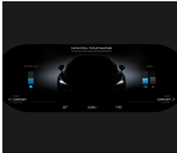
The welcome screen shows the time, outside temperature, odometer reading, 12V battery level, HV battery level and fuel gauge, selected powertrain and handling modes, and comfort entry on the Driver Display.
