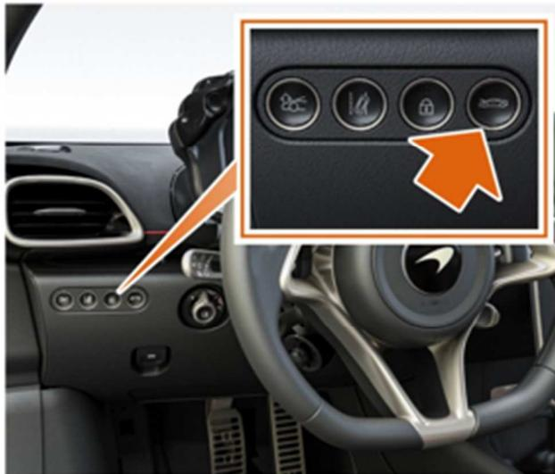
Alternatively, press and hold the dashboard button to fully unlock and slightly open the luggage compartment.
