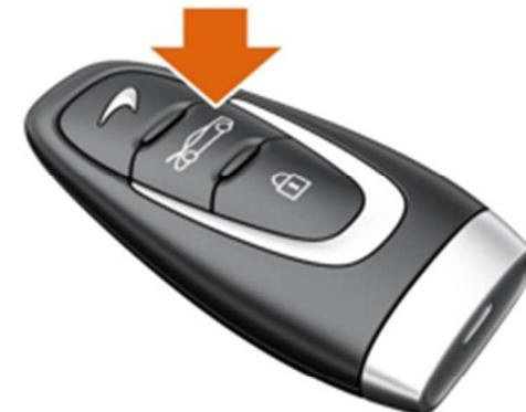
Press and hold the luggage release button on the key fob, the luggage compartment will fully unlock and open slightly.
