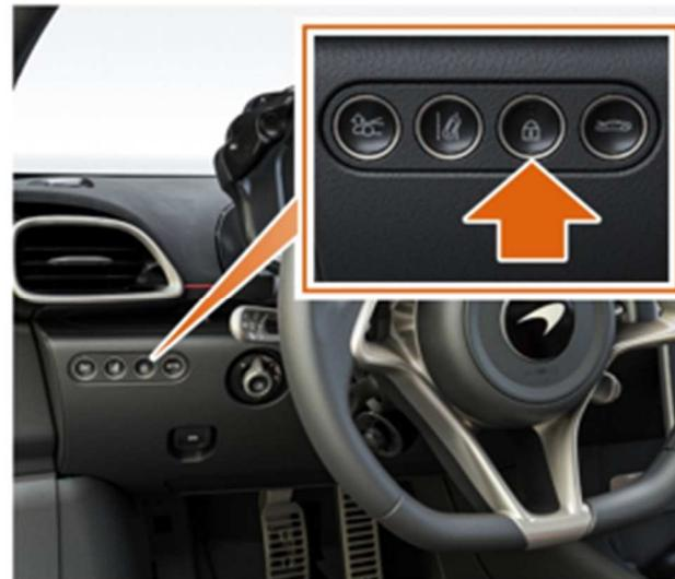
1. Press the central locking button to lock the vehicle, the light in the button will illuminate to indicate that the vehicle is locked. A door can be opened from inside the vehicle.
