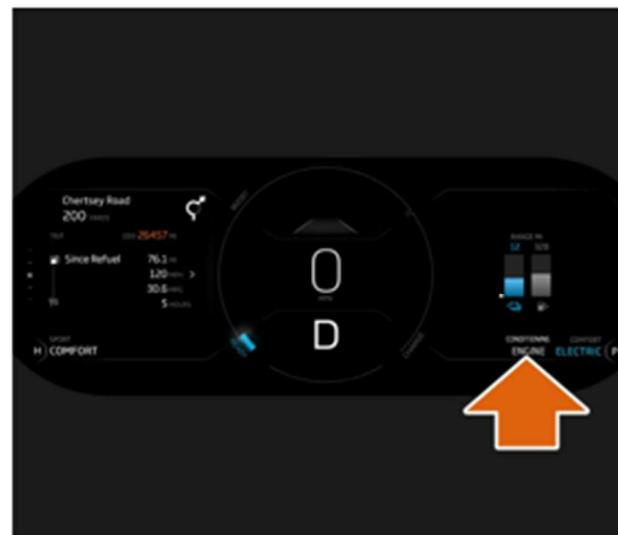
If the engine starts because electric range is depleted, the engine will provide drive to the wheels once the catalysts are warm. However, torque will be limited to that provided by the eMotor and the HV battery level will be sustained. A message displays recommending that you change powertrain mode.
