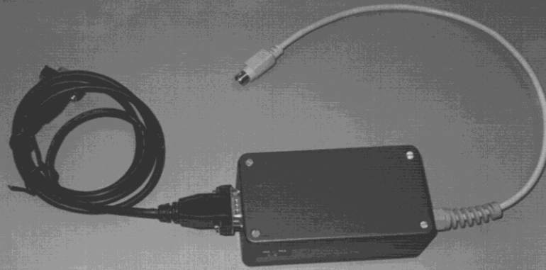
Ref: FCC ID N5 RP-FP-PL EA 92153 Interactive Displays Limited Controller box containing circuit board inc. serial cable to computer mini din connection to touchscreen.
