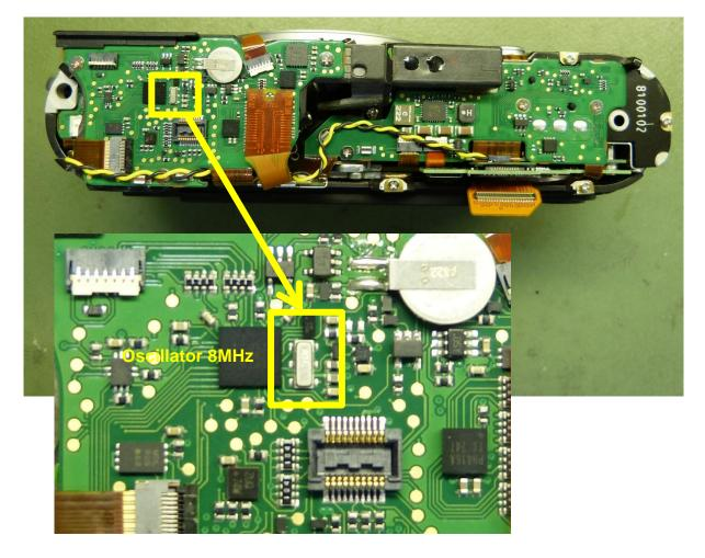
Photos Elec. Assembly – LEICA - Model 9217 STRICTLY CONFIDENTIAL
