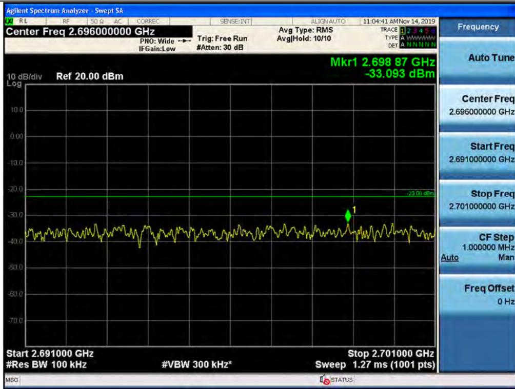
Spurious / BRS/EBS / Downlink / LTE 20 MHz / Middle / High Edge + 11 MHz ~ 10 GHz
