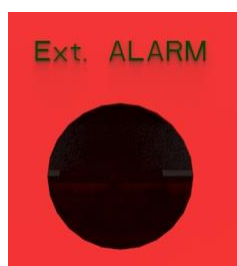
Figure 3-6 External Alarm Cutout Hole (0.87 in)
