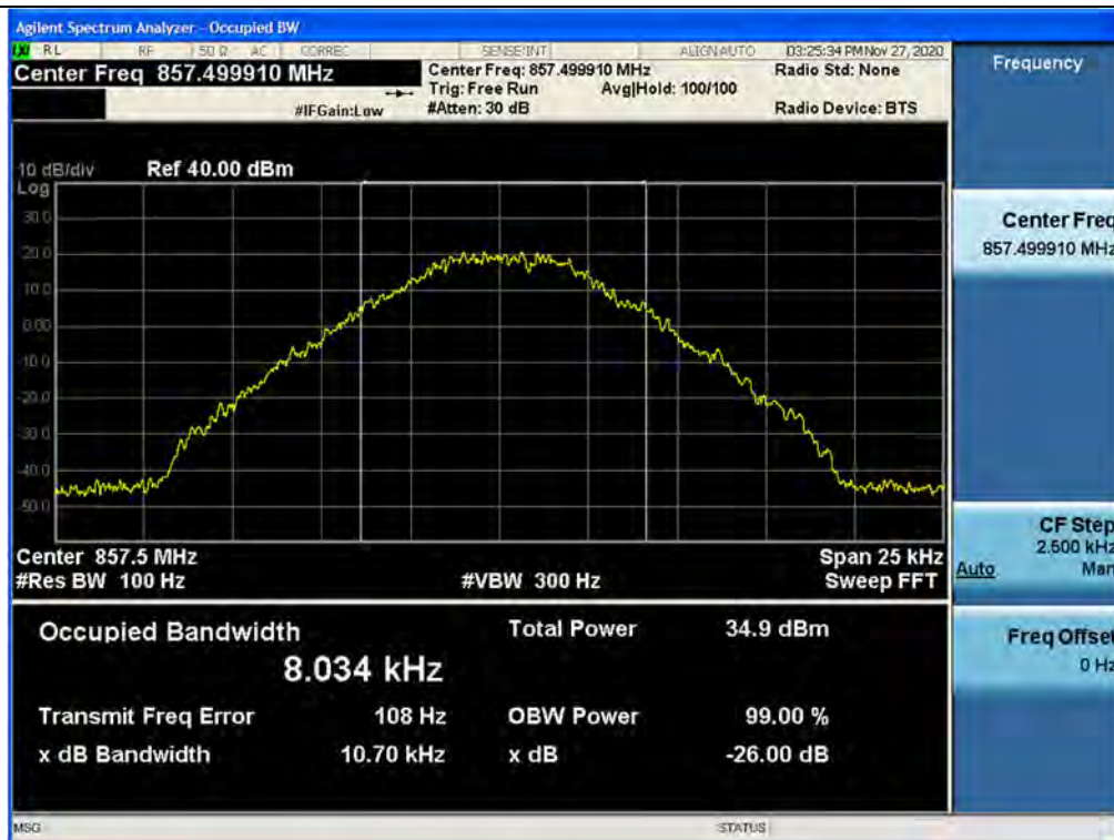
3 dB above the AGC threshold output / SMR / Downlink / P25 Phase 1
