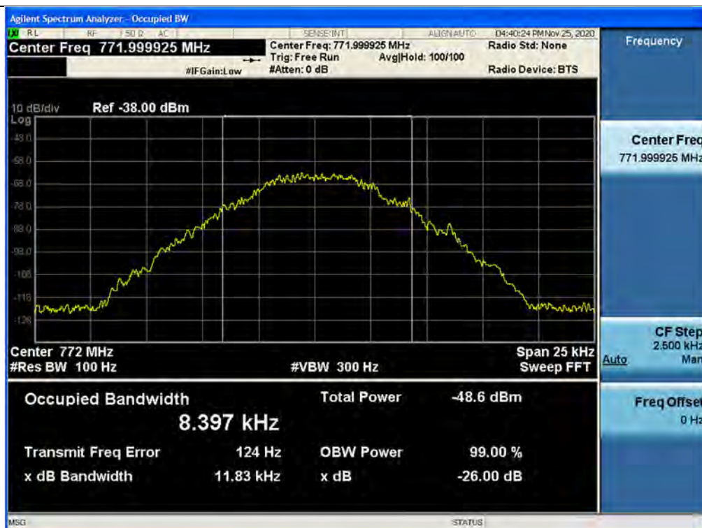
3 dB above the AGC threshold Input / PS Narrowband / Downlink / P25 Phase 1
