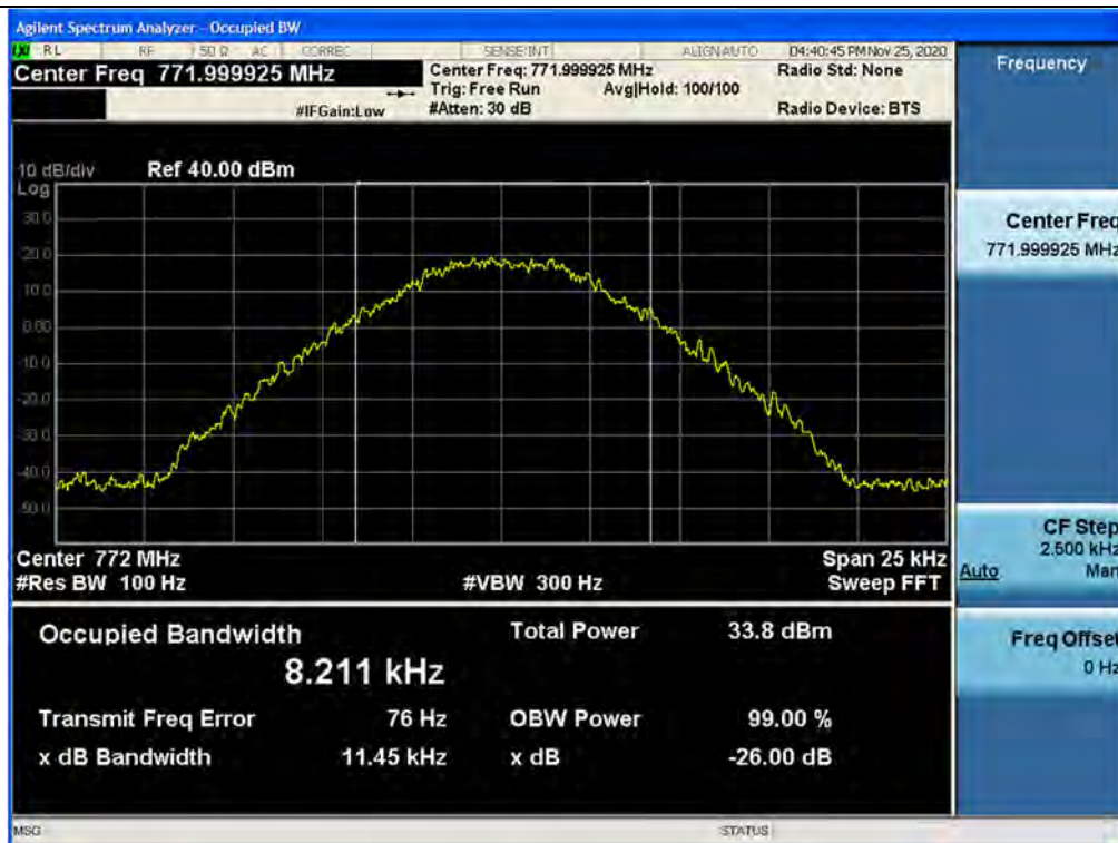
3 dB above the AGC threshold output / PS Narrowband / Downlink / P25 Phase 1
