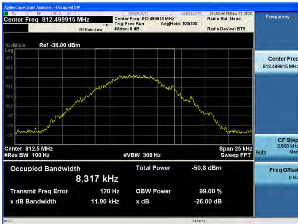
3 dB above the AGC threshold Input / SMR / Uplink / P25 Phase 1
