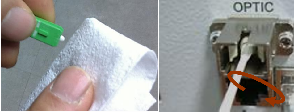
Figure 3-17 Optic Connector Cleaning (left) and Optic Port Cleaning (right)
