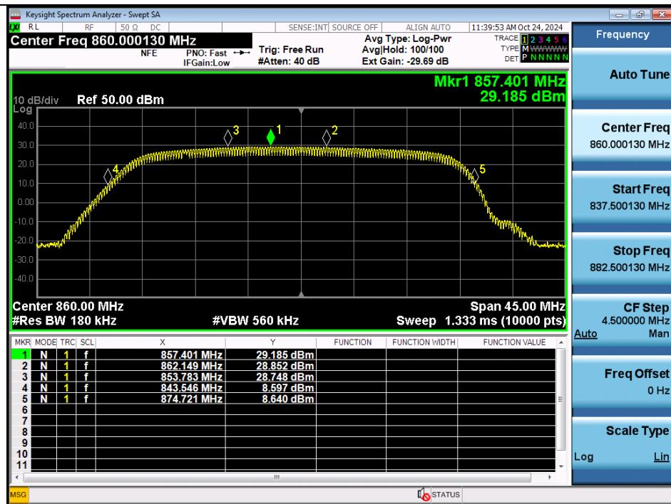
**Note:** The EUT is amplified in multiple 800 MHz bands, but this test report uses the results for the frequency range of 851 ~ 854 MHz, 854 ~ 861 MHz, 862 ~ 869 MHz.
