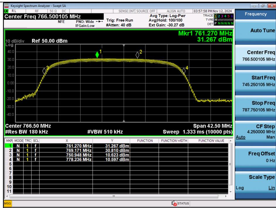
**Note:** The EUT is amplified in multiple 700 MHz bands, but this test report uses the results for the frequency range of 769 ~ 775 MHz.
