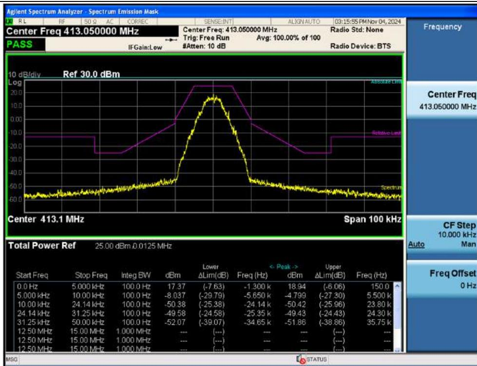
3 dB above the AGC threshold Input / UHF (406.1 ~ 420) / Downlink / P25 Phase 1 / Mask C
