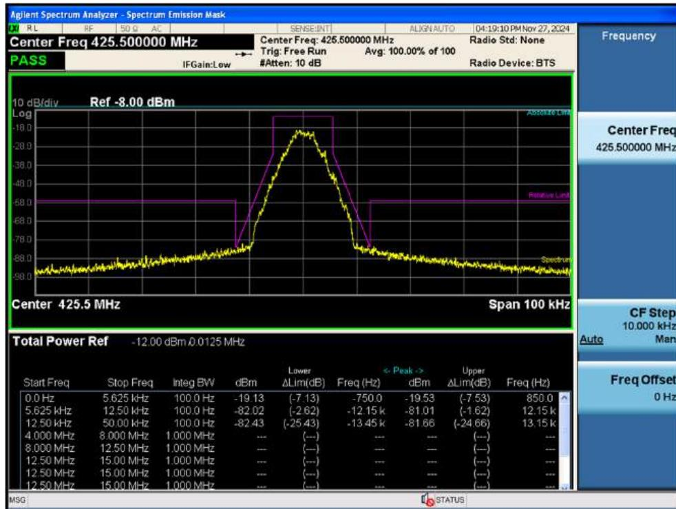
3 dB above the AGC threshold output / UHF (421 ~ 430.0) / Downlink / P25 Phase 1 / Mask D
