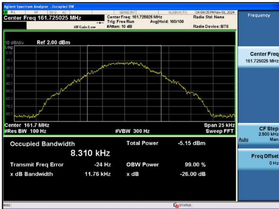
3 dB above the AGC threshold output / VHF (150.05 ~ 173.4) / Downlink / P25 Phase 1
