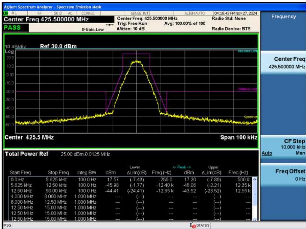
3 dB above the AGC threshold Input / UHF (421 ~ 430.0) / Downlink / P25 Phase 1 / Mask D
