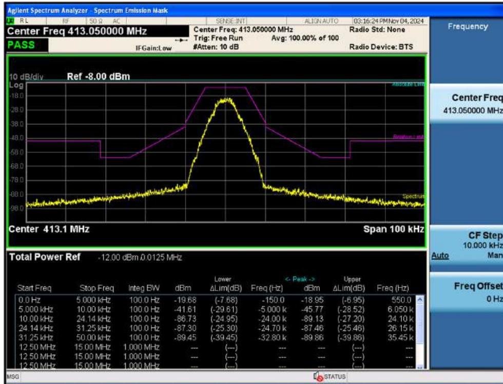
3 dB above the AGC threshold output / UHF (406.1 ~ 420) / Downlink / P25 Phase 1 / Mask C
