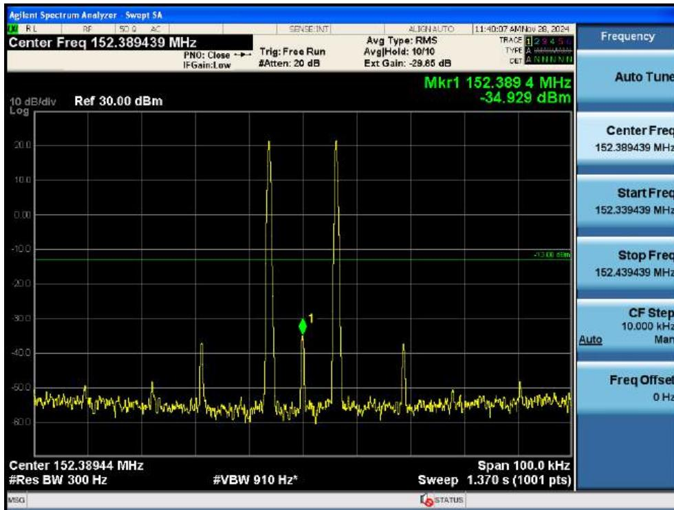
3 dB above the AGC threshold Out-of-band (two adjacent test signals) / VHF (150.05 ~ 173.4) / Downlink
