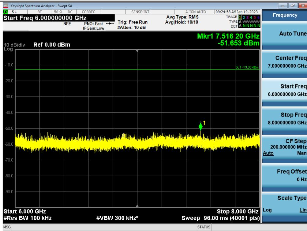
Spurious / Simultaneous(700LU\_LTE+LTE) / Downlink / 763 MHz ~ 775 MHz
