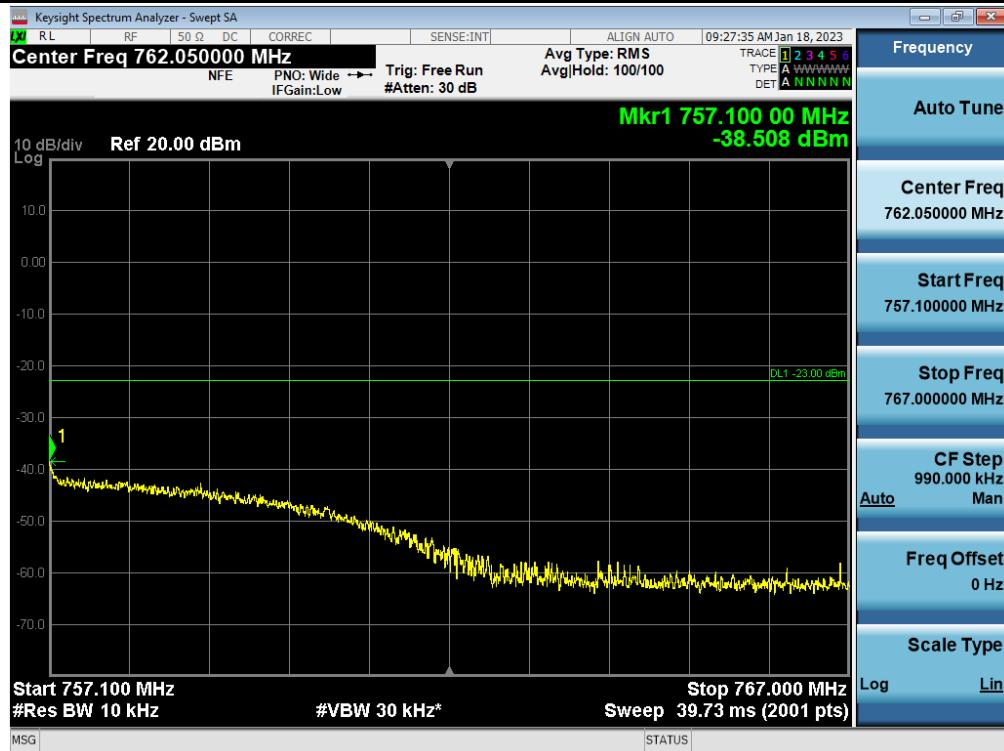
Spurious / Upper 700 MHz / Downlink / LTE 10 MHz / Low / High Edge + 10 MHz ~ 2 GHz
