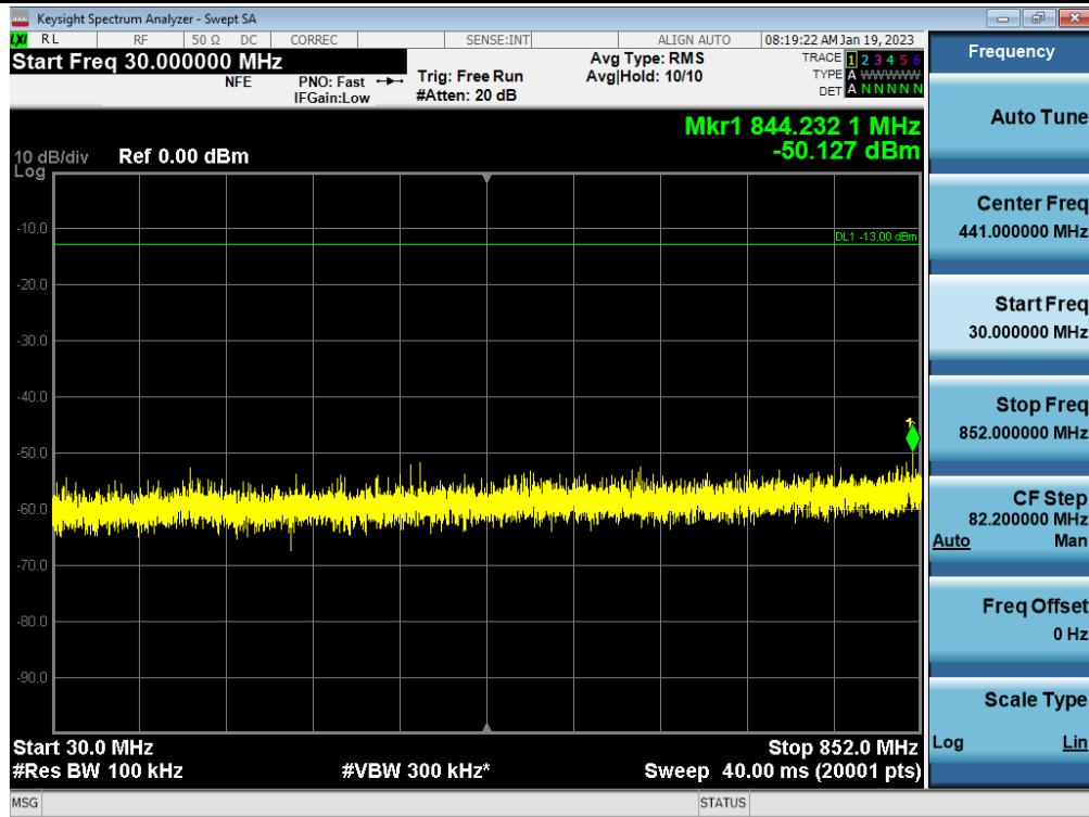
Spurious / Simultaneous (ESMR+Cellular\_NR+LTE) / Downlink / 852 MHz ~ 861.7 MHz
