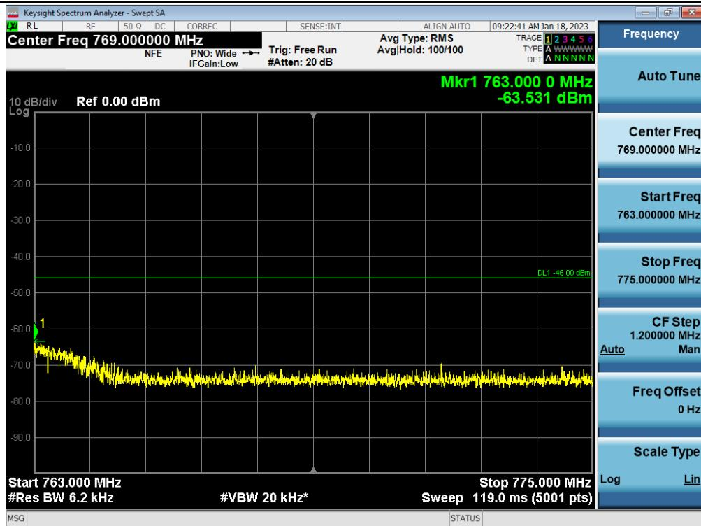
Spurious / Upper 700 MHz / Downlink / LTE 10 MHz / Middle / 793 MHz ~ 805 MHz
