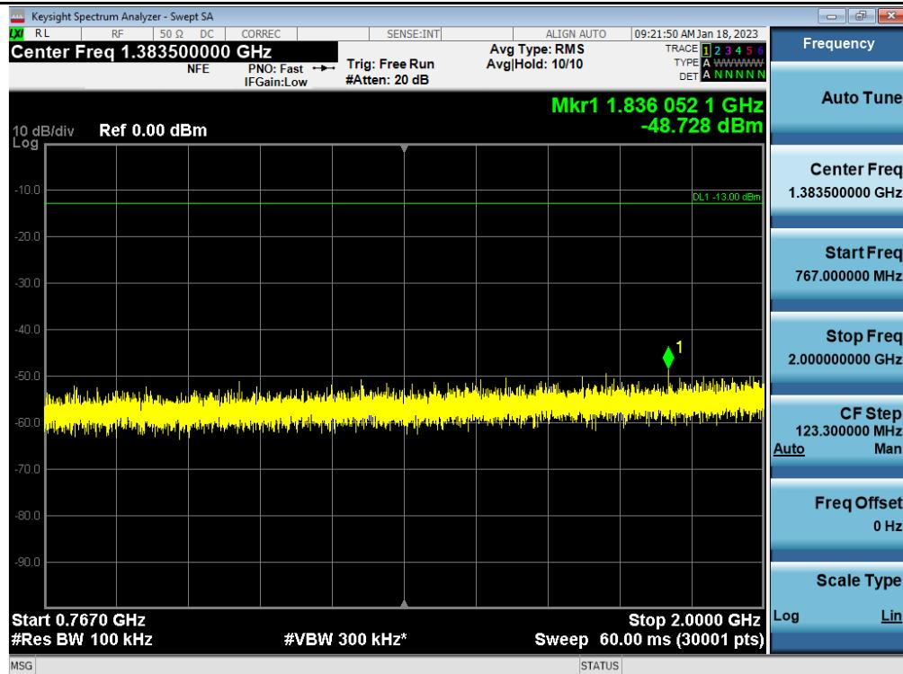
Spurious / Upper 700 MHz / Downlink / LTE 10 MHz / Middle / 2 GHz ~ 4 GHz
