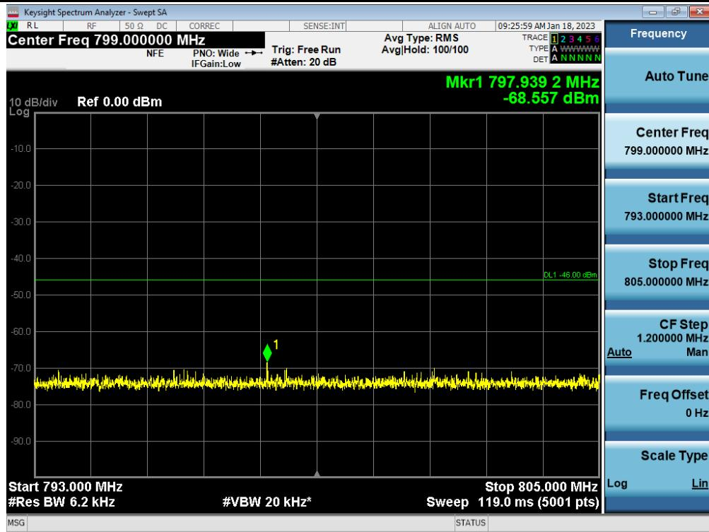
Spurious / Upper 700 MHz / Downlink / LTE 10 MHz / High / 1 559 MHz ~ 1 610 MHz
