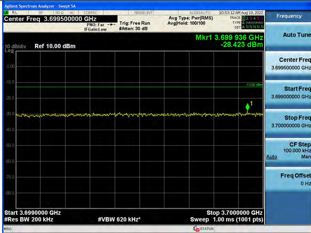
+3 dB above Out-of-band (single test signal) / C-Band / Downlink / 5G NR 20 MHz / Upper
