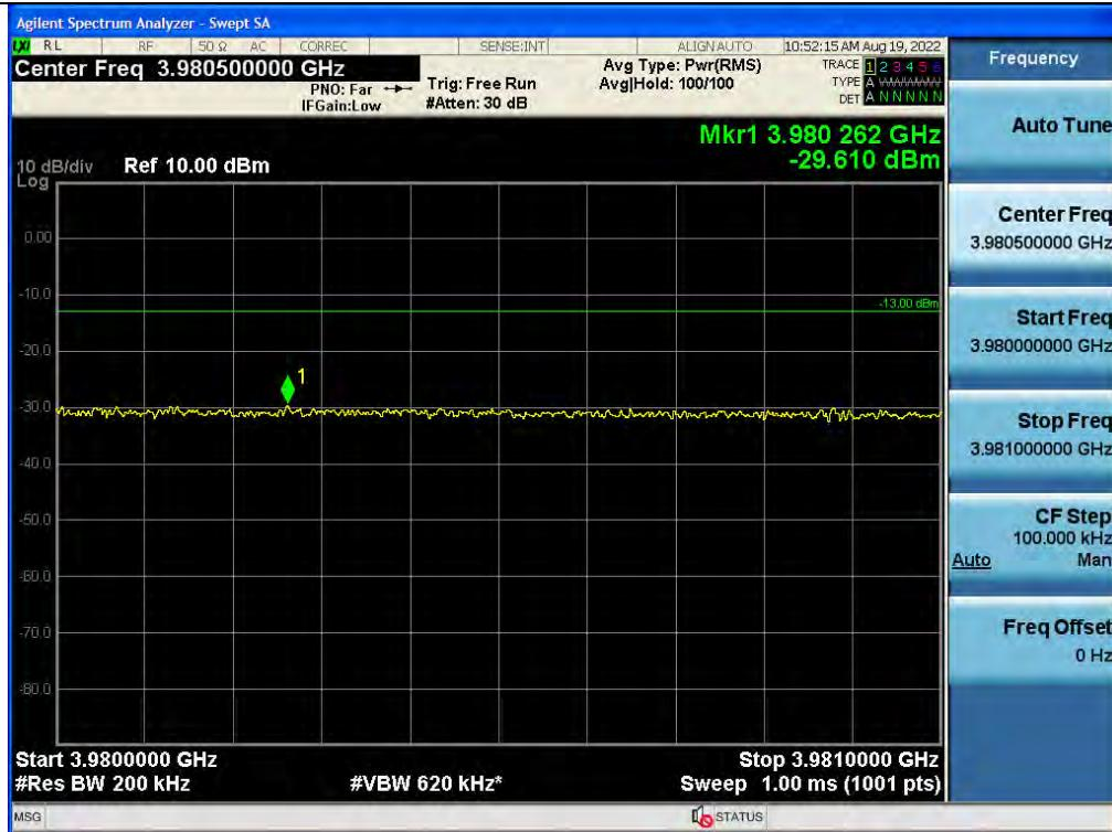
+3 dB above Out-of-band (single test signal) / C-Band / Downlink / 5G NR 20 MHz / Lower
