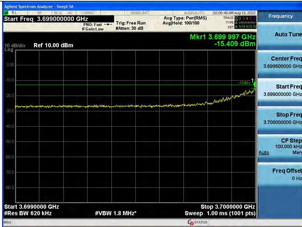
+3 dB above Out-of-band (single test signal) / C-Band / Downlink / 5G NR 60 MHz / Upper
