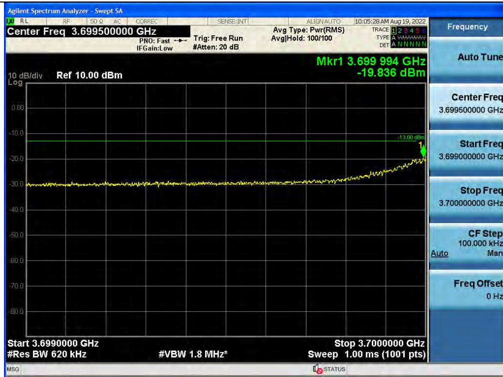
+3 dB above Out-of-band (two adjacent test signals) / C-Band / Downlink / 5G NR 60 MHz / Upper
