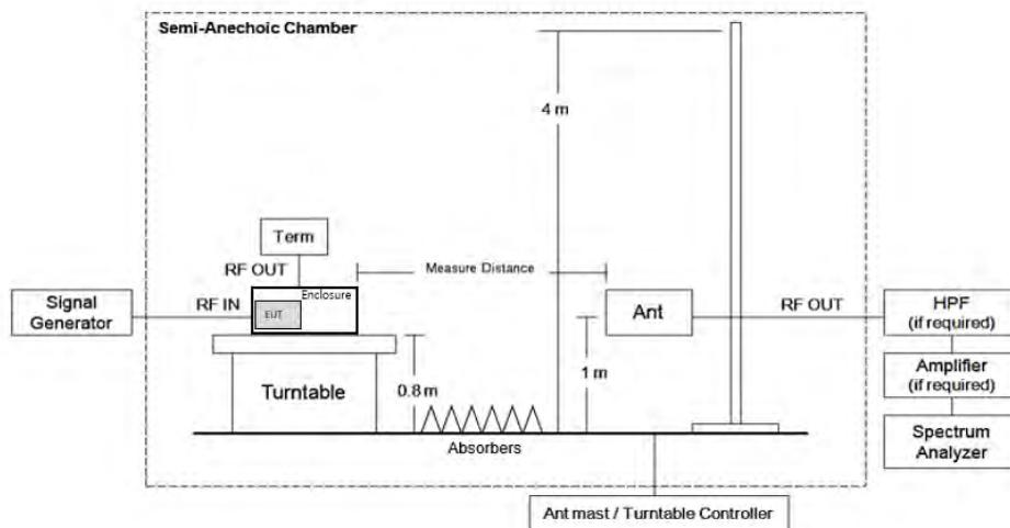
※ EUT position is adopted by placement of floor-standing refer to section 5.5.2.3.2 of ANSI C63.26-2015
