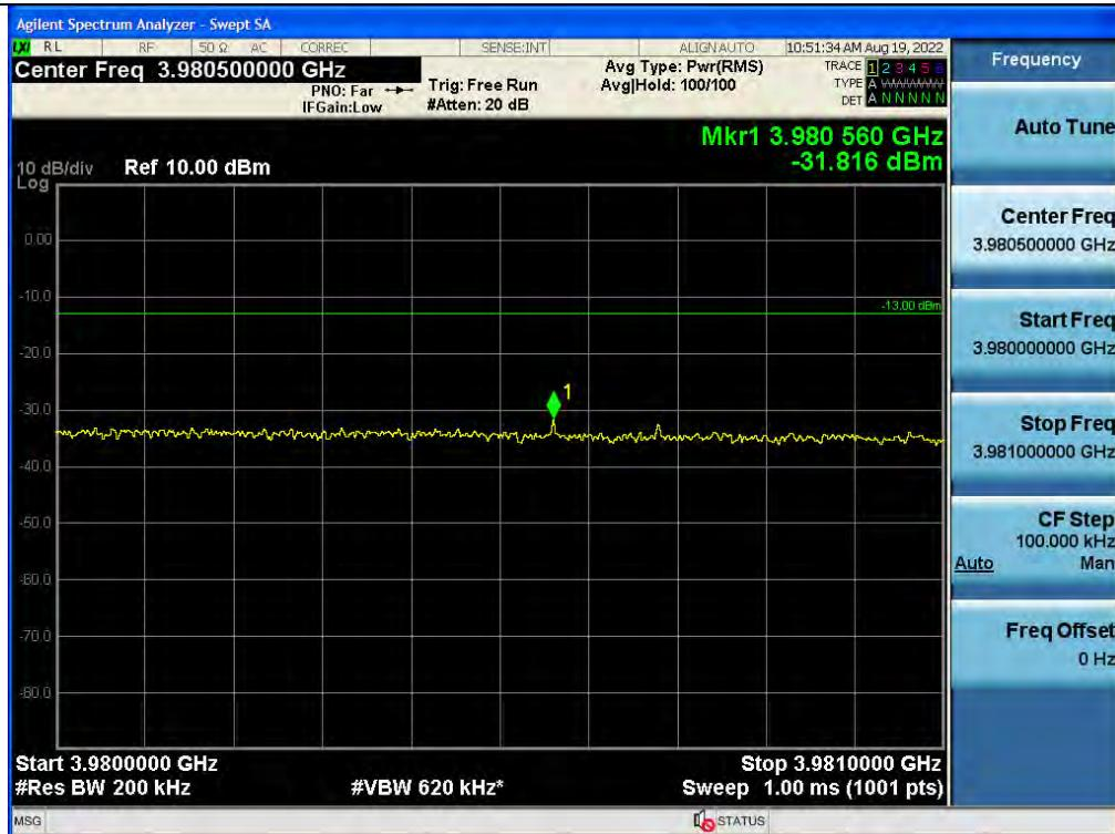
+3 dB above Out-of-band (two adjacent test signals) / C-Band / Downlink / 5G NR 20 MHz / Lower
