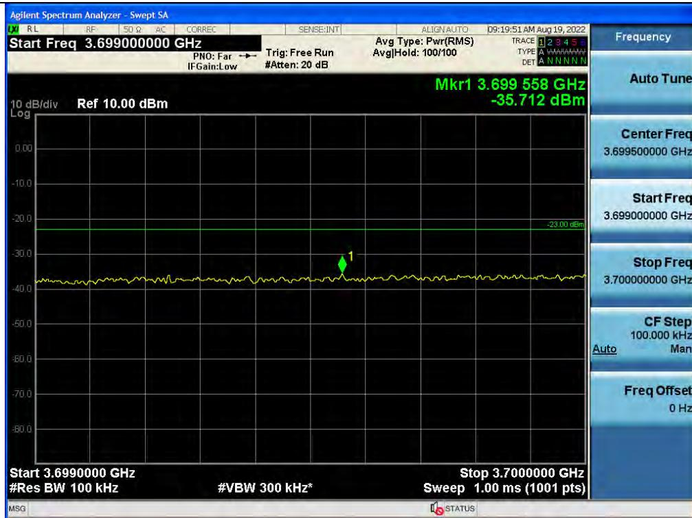
+3 dB above Out-of-band (single test signal) / C-Band / Downlink / 5G NR 100 MHz / Upper
