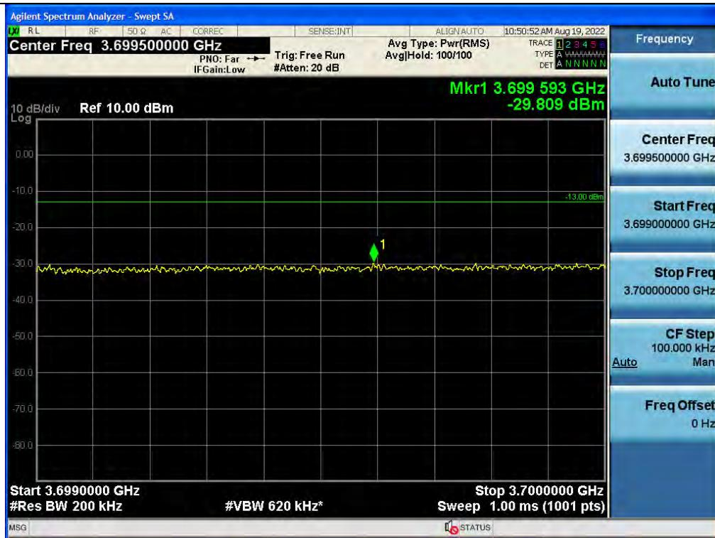
Out-of-band (two adjacent test signals) / C-Band / Downlink / 5G NR 20 MHz / Upper
