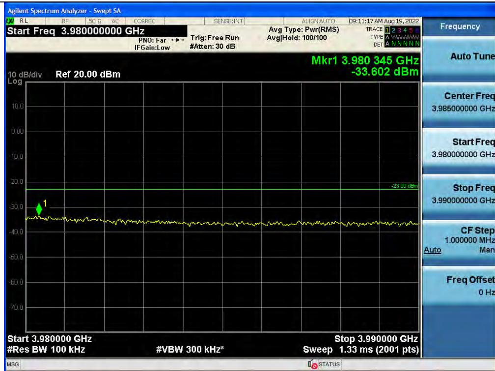
Spurious / C-Band / Downlink / 5G NR 80 MHz / Low / High Edge + 10 MHz ~ 10 GHz
