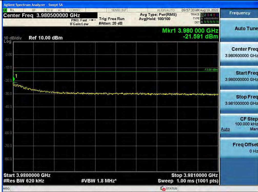
+3 dB above Out-of-band (two adjacent test signals) / C-Band / Downlink / 5G NR 60 MHz / Lower
