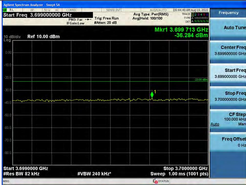
+3 dB above Out-of-band (single test signal) / C-Band / Downlink / 5G NR 80 MHz / Upper
