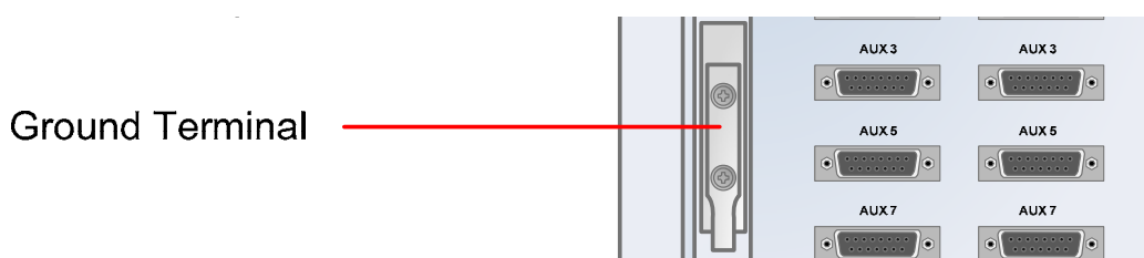
Figure 6-3 HE Ground Cable Connection, Protective Earthing Conductor (HE chassis rear side)
