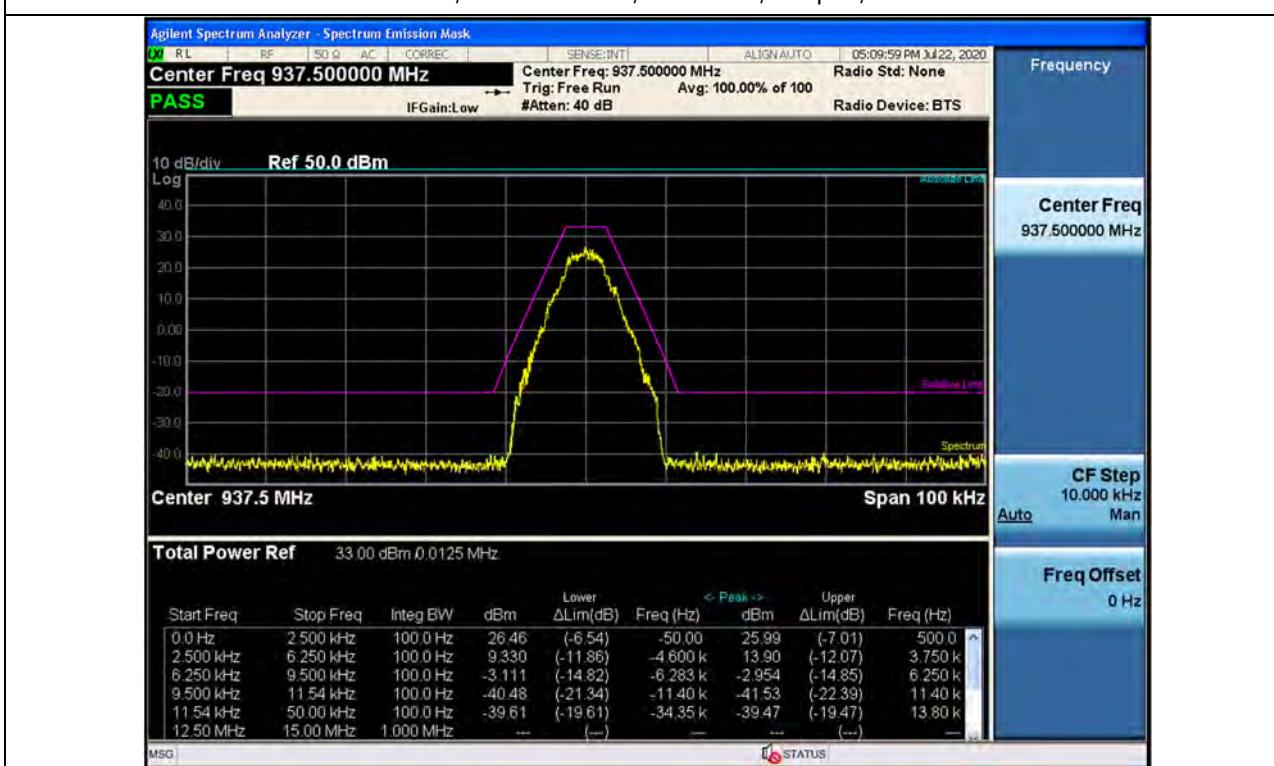
Emission Mask / 935 ~ 940 MHz / Downlink / +3 dB Output / P25 Phase 1
