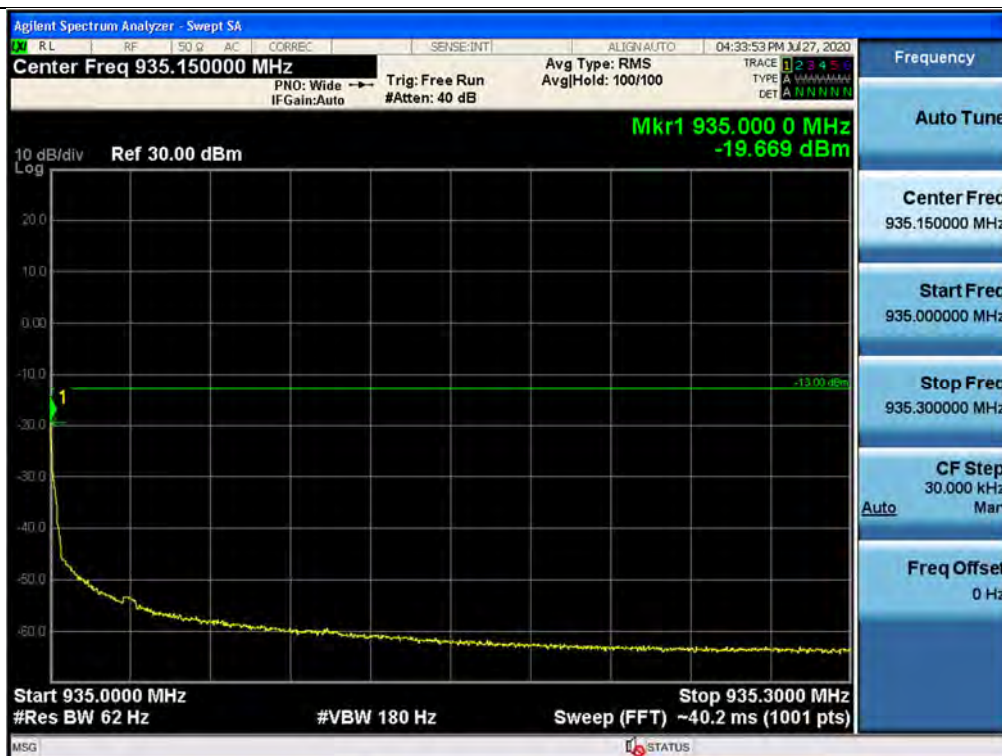
Out-of-band (single test signals) / 932 ~ 935 MHz / Downlink / P25 Phase 2 / Upper
