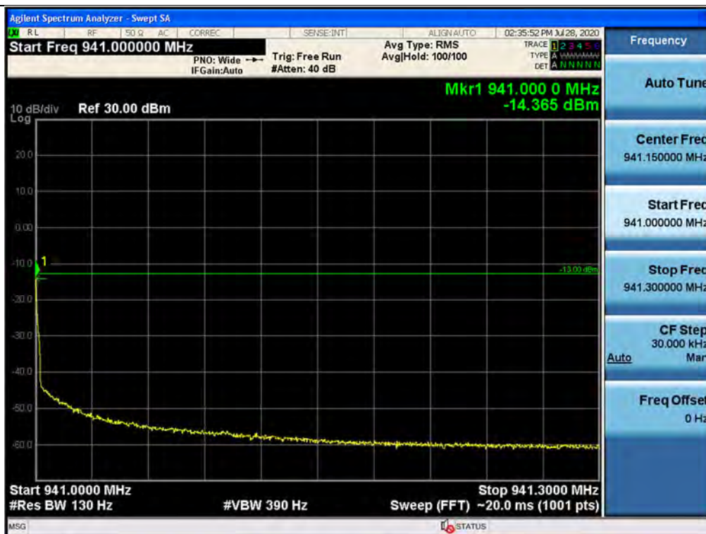
Out-of-band (single test signals) / 940 ~ 941 MHz / Downlink / P25 Phase 1 / Upper
