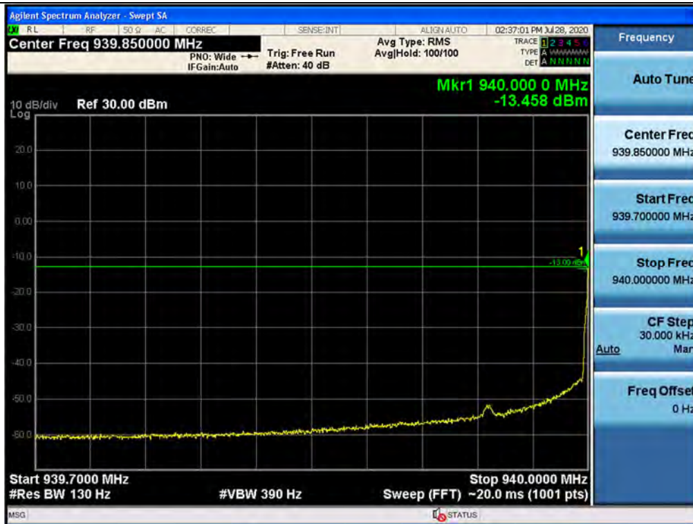
Out-of-band (single test signals) / 940 ~ 941 MHz / Downlink / P25 Phase 1 / Lower
