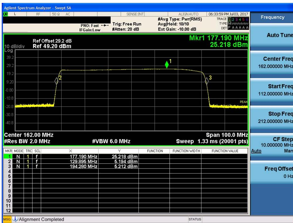
\* This device must be used with a duplexer by the user, and can be used with external filters. This test results were measured without duplexer or external filters. So, the test results were measured to be about  $\pm 250$  % of each pass band from the center frequency according to the test procedure.
