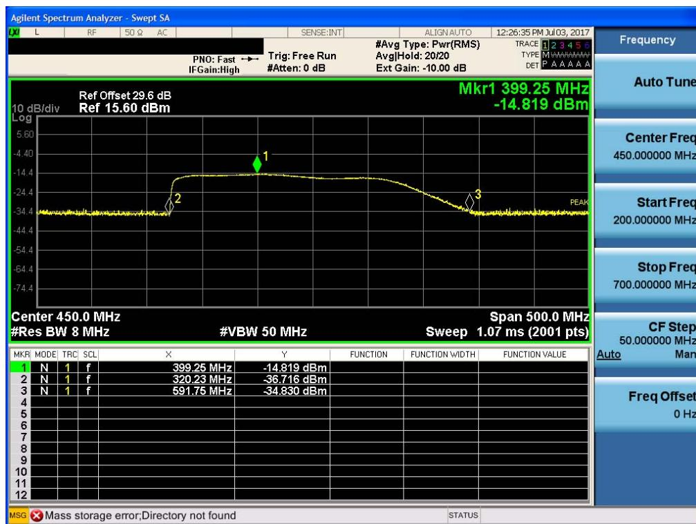
\* This device must be used with a duplexer by the user, and can be used with external filters. This test results were measured without duplexer or external filters. So, the test results were measured to be about  $\pm 250$  % of each pass band from the center frequency according to the test procedure.
