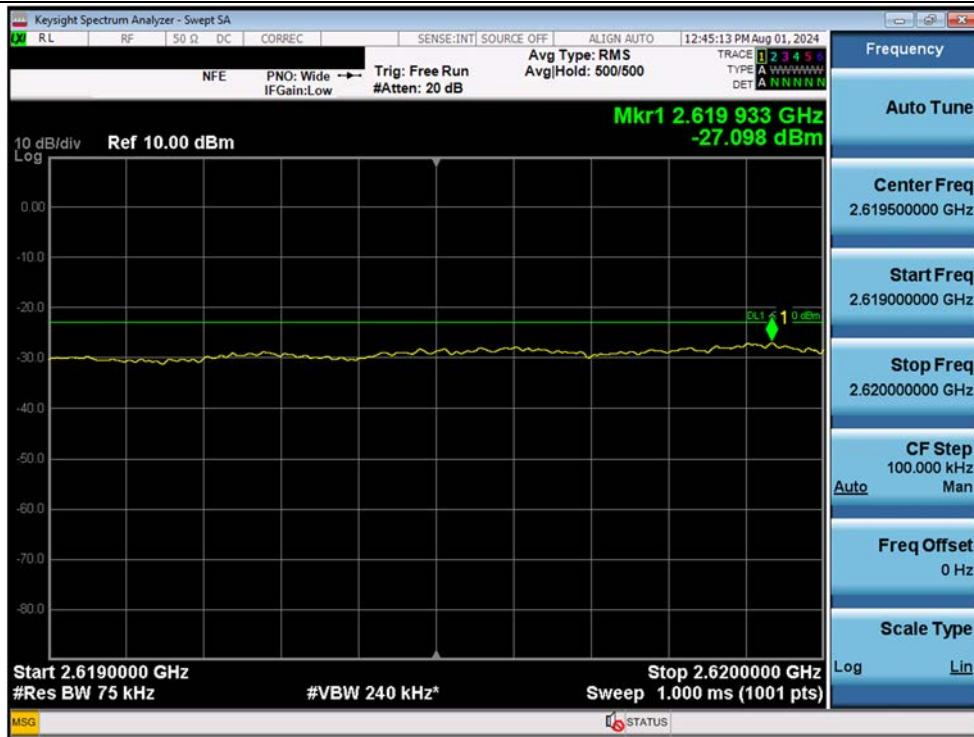
+3 dB above Out-of-band (single test signal) / BRS/EBS / Downlink / 5G NR 70 MHz / Upper
