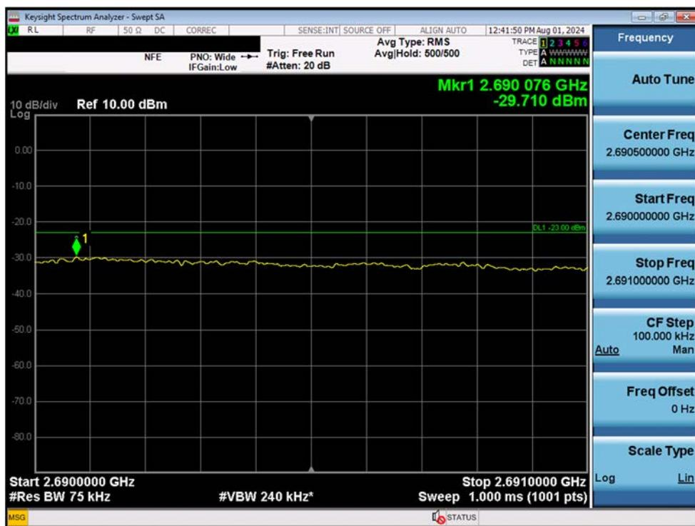
+3 dB above Out-of-band (single test signal) / BRS/EBS / Downlink / 5G NR 70 MHz / Lower
