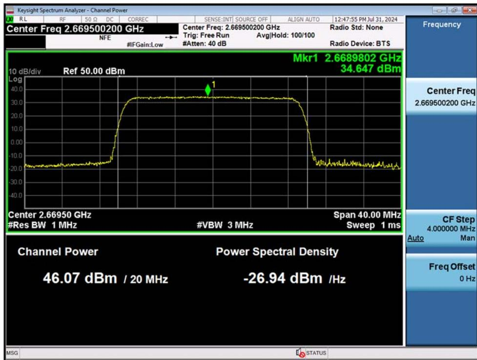
3 dB above the AGC threshold PSD / BRS/EBS / Downlink / LTE 20 MHz
