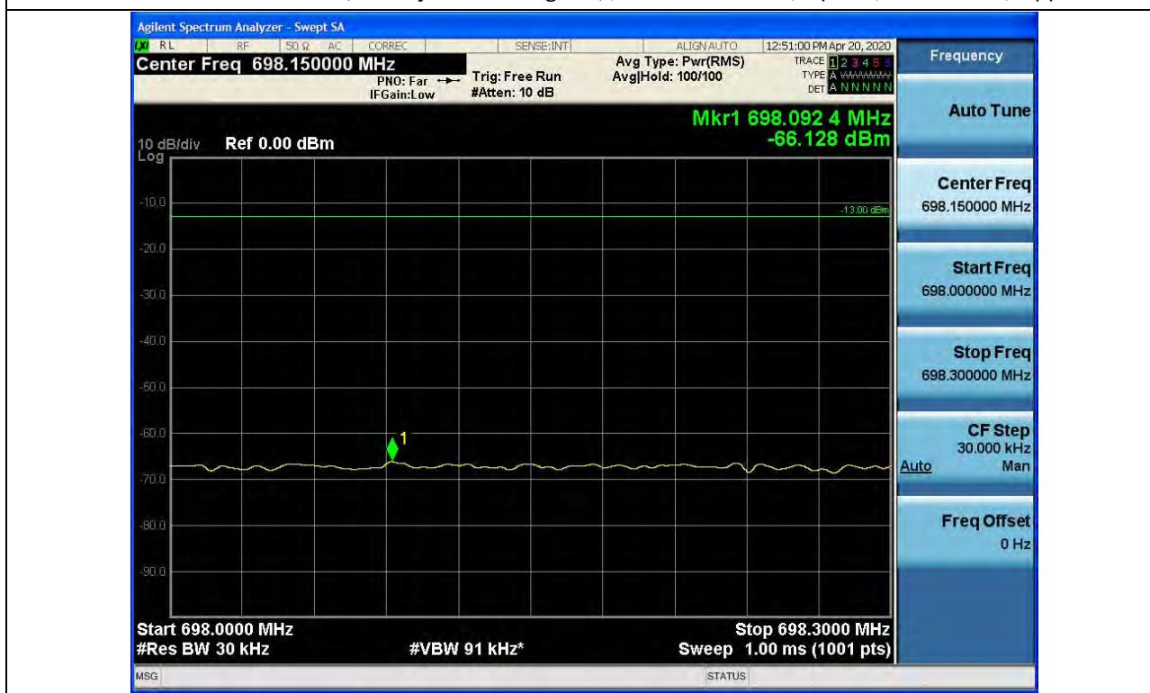
+3 dB above Out-of-band (two adjacent test signals) / 600 MHz Service / Uplink / LTE 20 MHz / Lower
