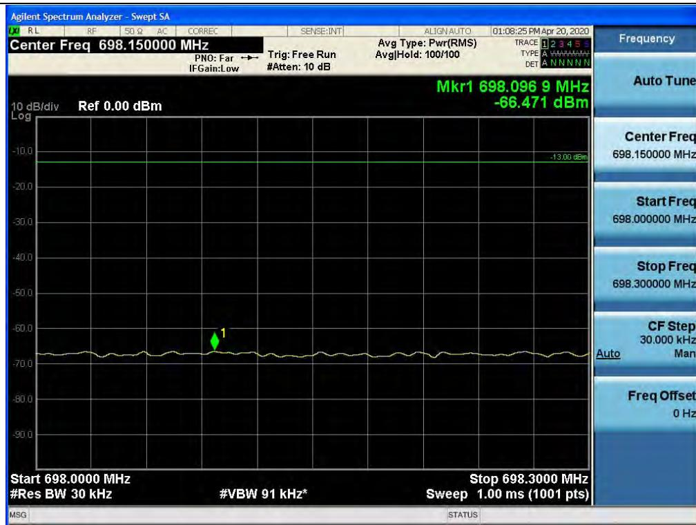
+3 dB above Out-of-band (single test signals) / 600 MHz Service / Uplink / 5G NR 20 MHz / Lower
