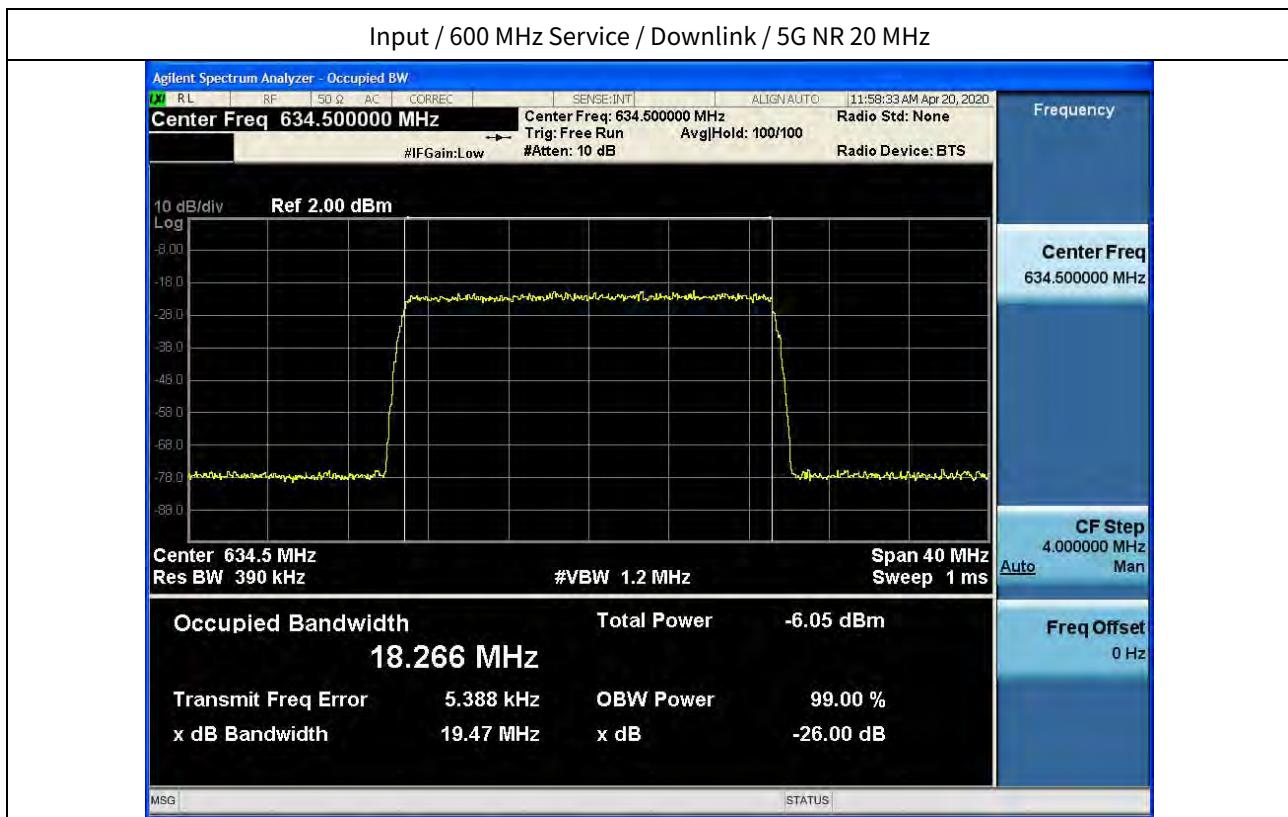
3 dB above the AGC threshold output / 600 MHz Service / Downlink / 5G NR 20 MHz
