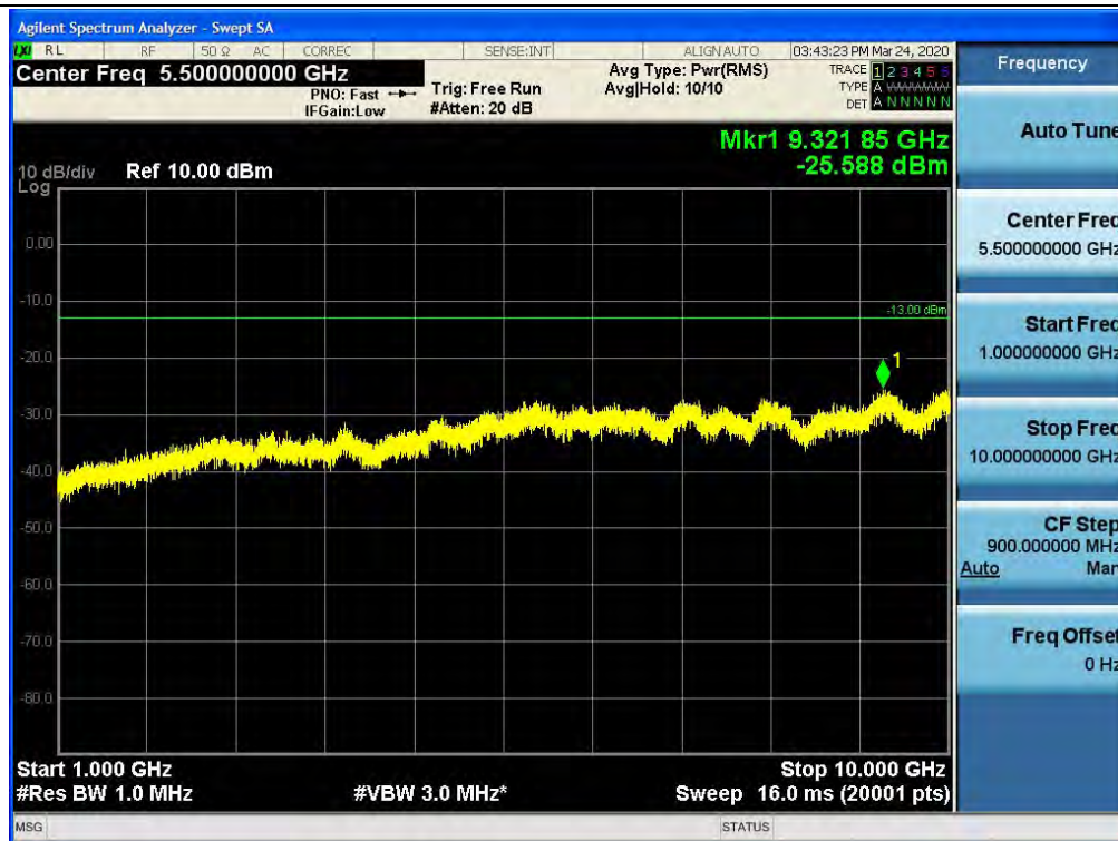
Spurious / Cellular / Uplink / LTE 20 MHz / Middle / 1 GHz ~ 10 GHz
