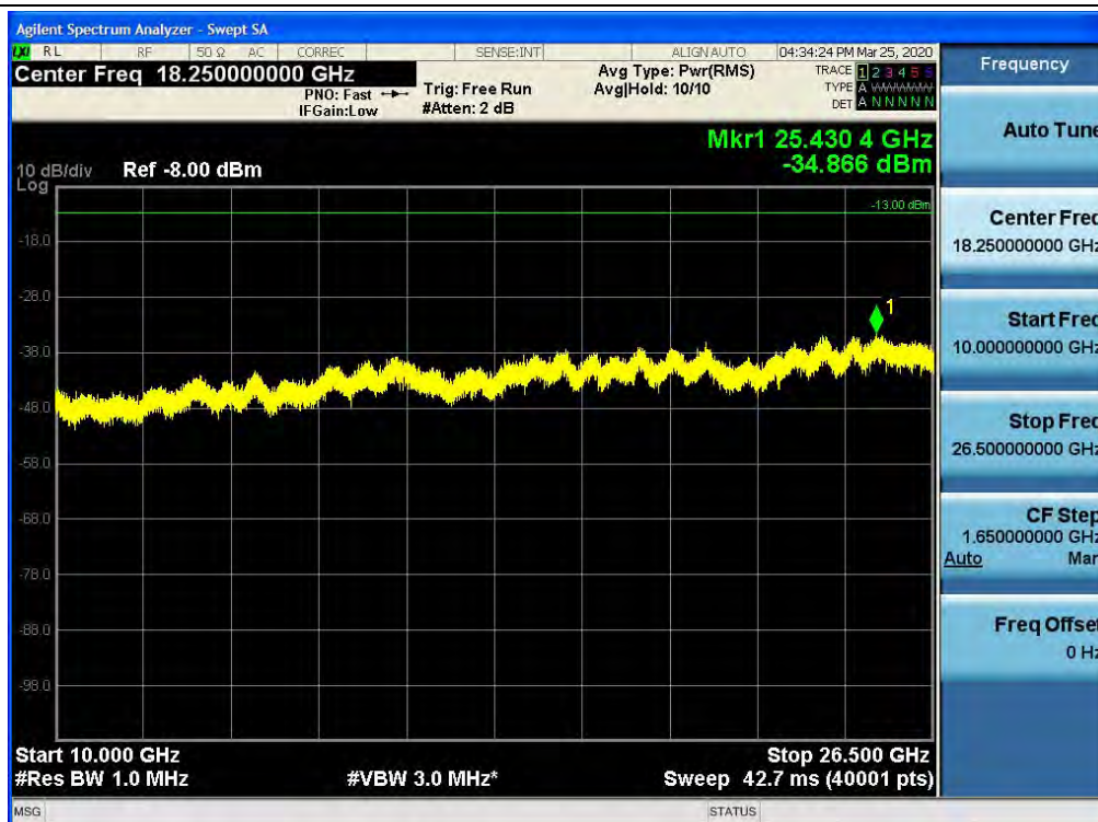
Spurious / BRS/EBS / Uplink / LTE 20 MHz / Low / 10 GHz ~ 26.5 GHz
