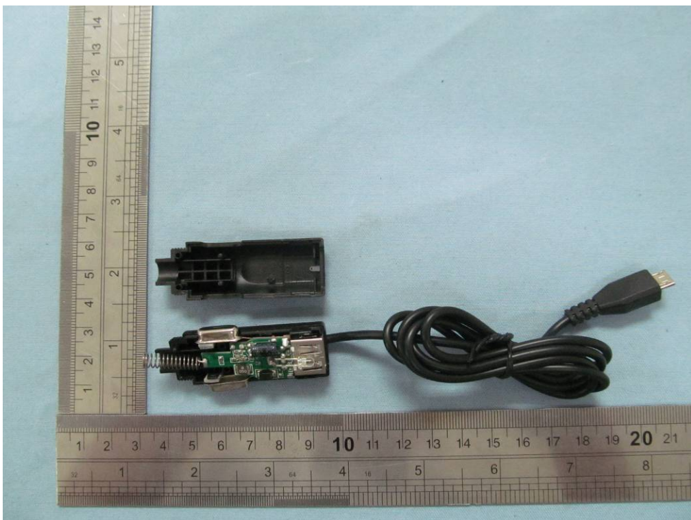
OPEN VIEW OF VEHICLE CHARGER
