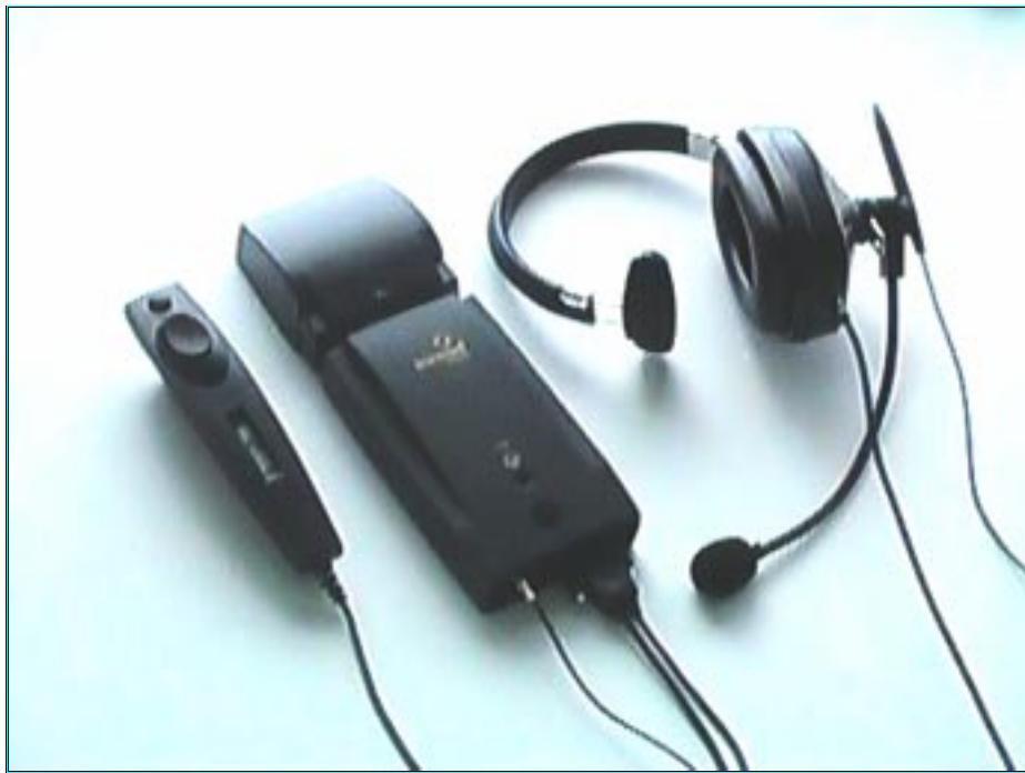
The Inroad Inquire wearable computer is a voice-activated, wearable, wireless information access device made up of the following components:
