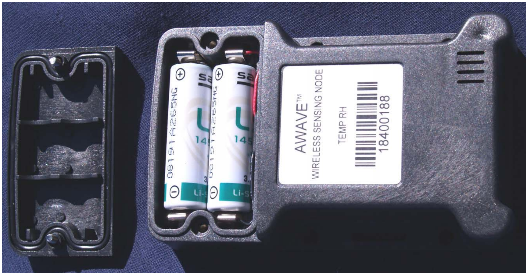
Photo 1: Phase IV Engineering – AWAVE – WSN – Battery door removed
