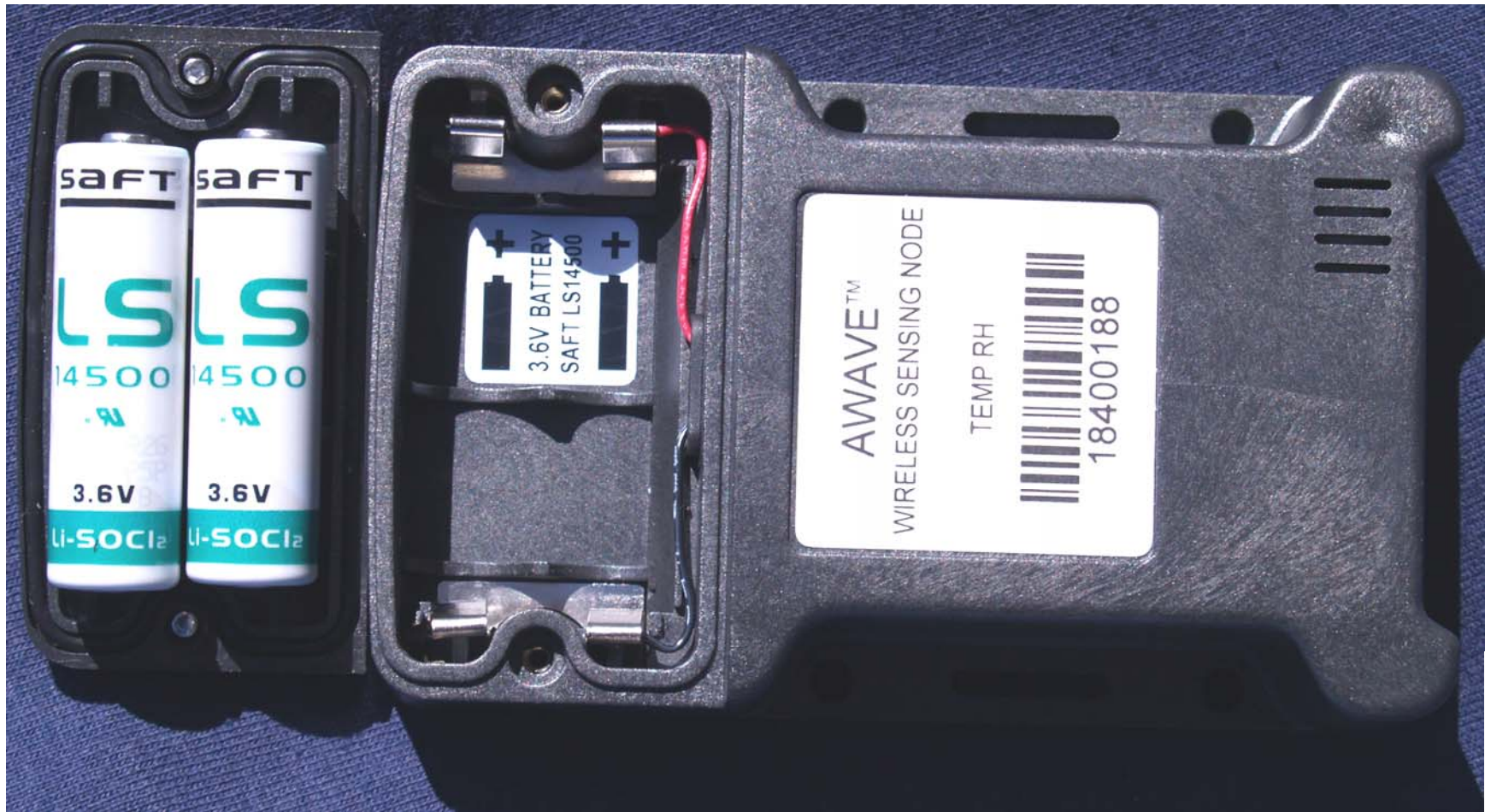
Photo 2: Phase IV Engineering – AWAVE – WSN – Batteries on battery door
