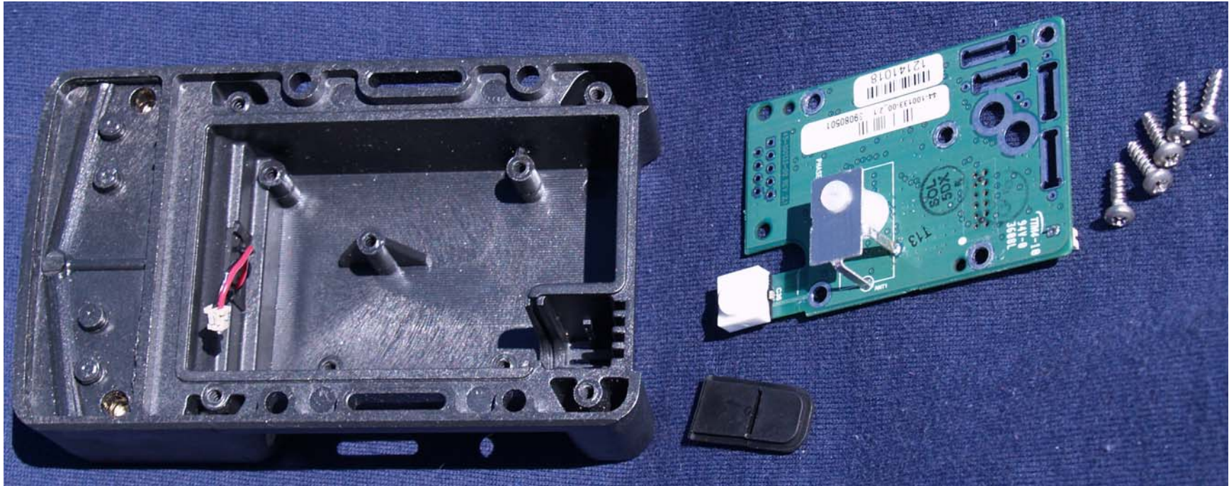
Photo 5: Phase IV Engineering – AWAVE – WSN – PCB Removed
