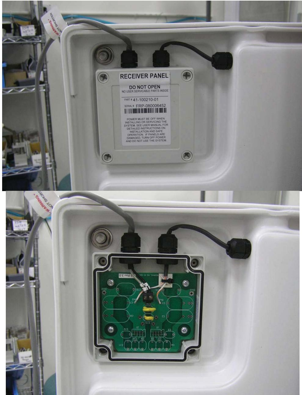
**Circuit Board in Receiver Panel with cover on and cover off.**
