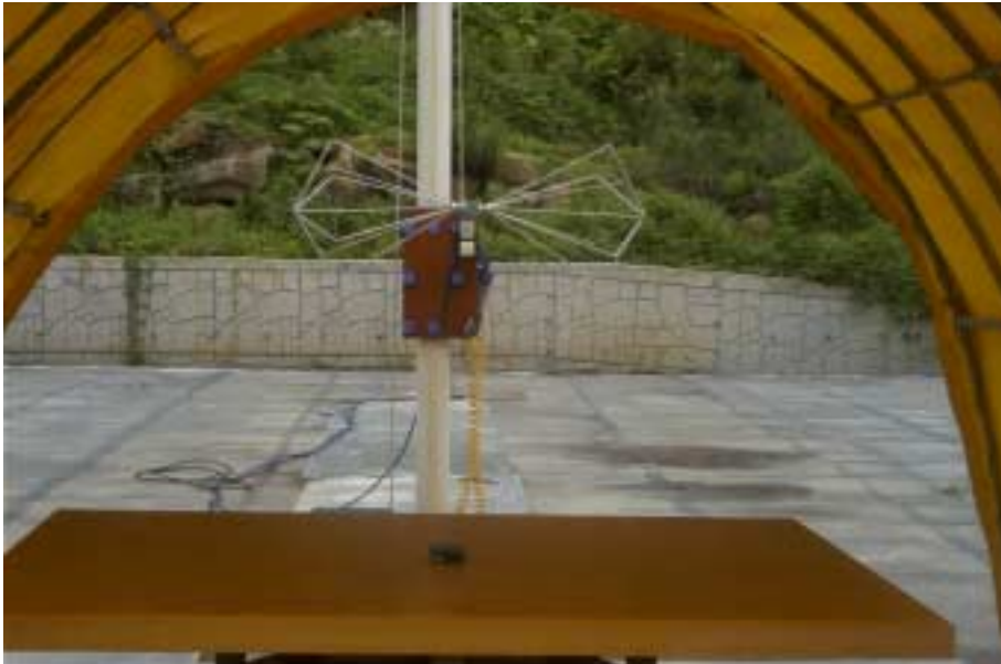
Photograph 1 : Setup for radiated Emissions
