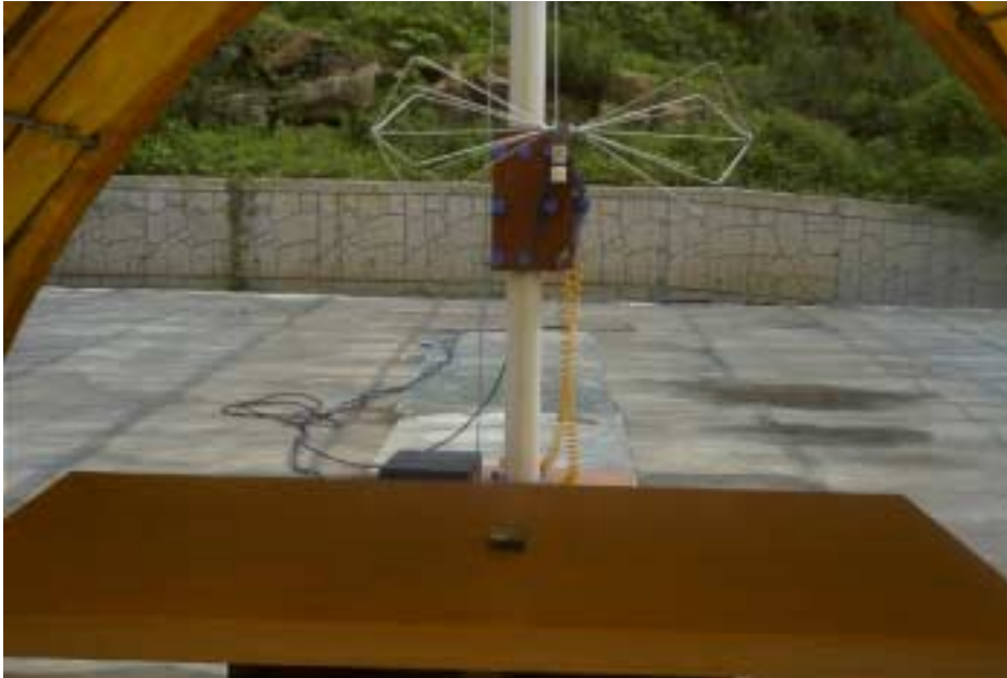
Photograph 1 : Setup for radiated Emissions
