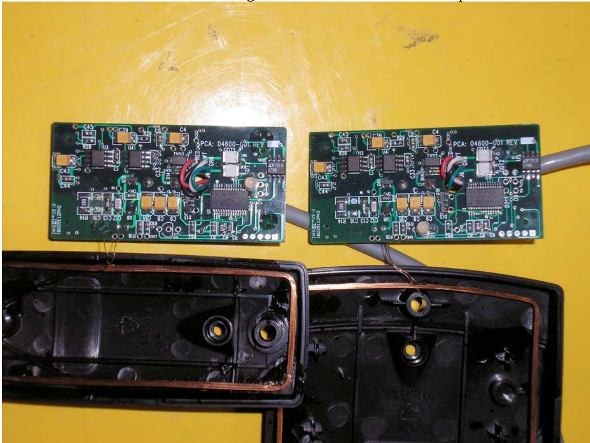
Detail NXT-1R and NXT-3R showing same PCB board, different loop antennas
