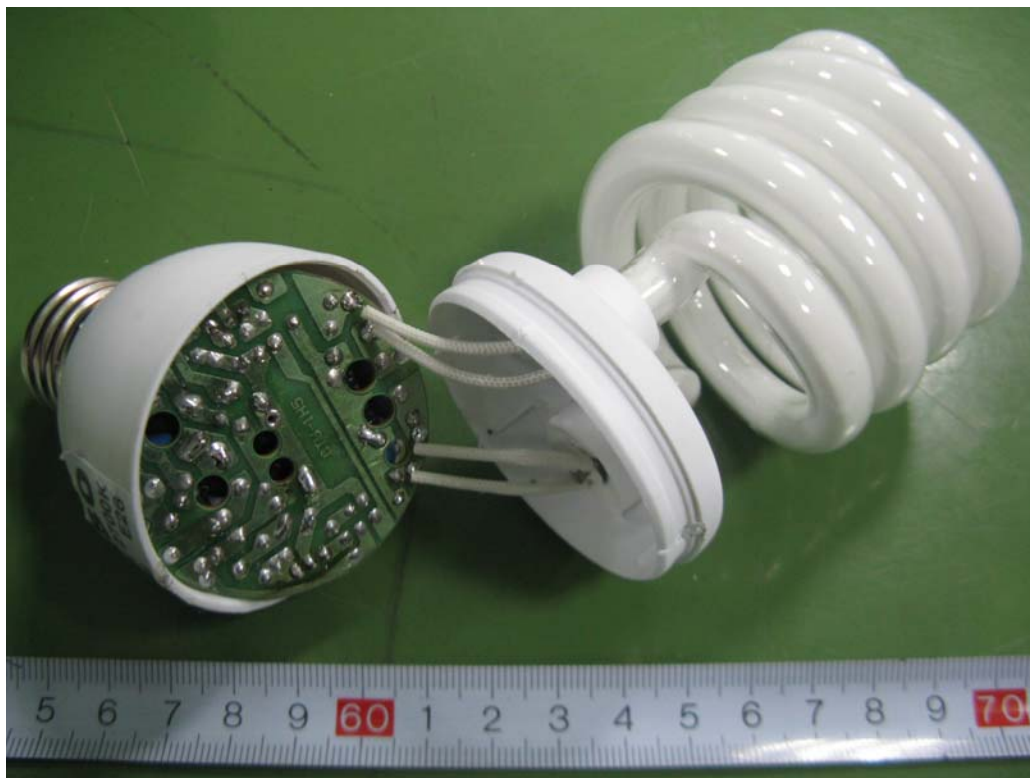
CMTL 25W: EUT - Cover off View
