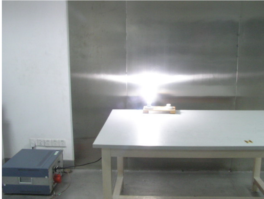
CPTL20W: Conducted Emissions - Front View
