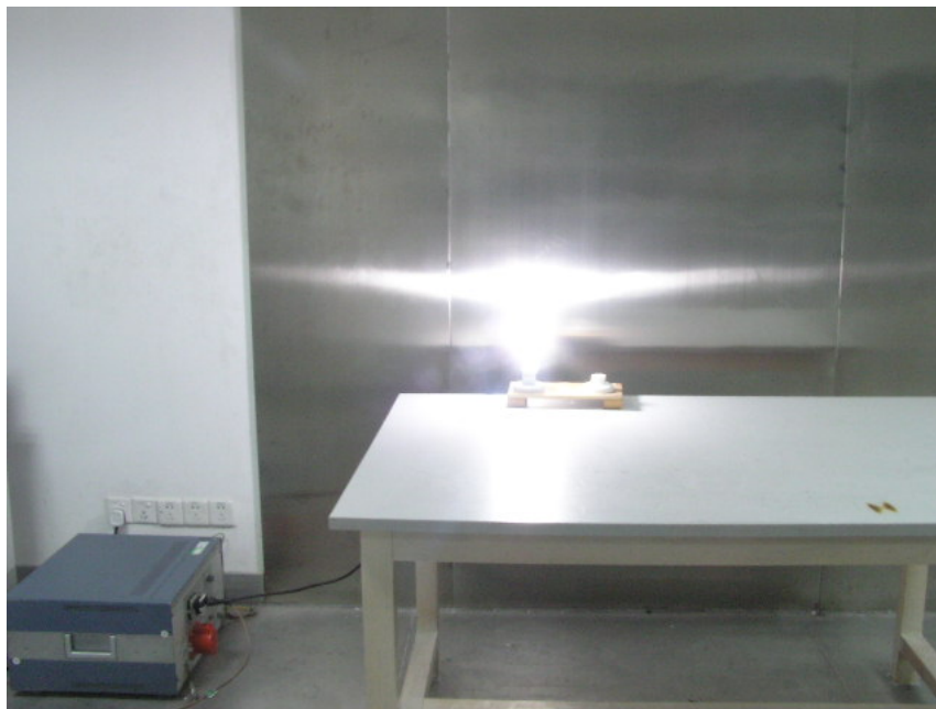
CPTL13W: Conducted Emissions - Front View
