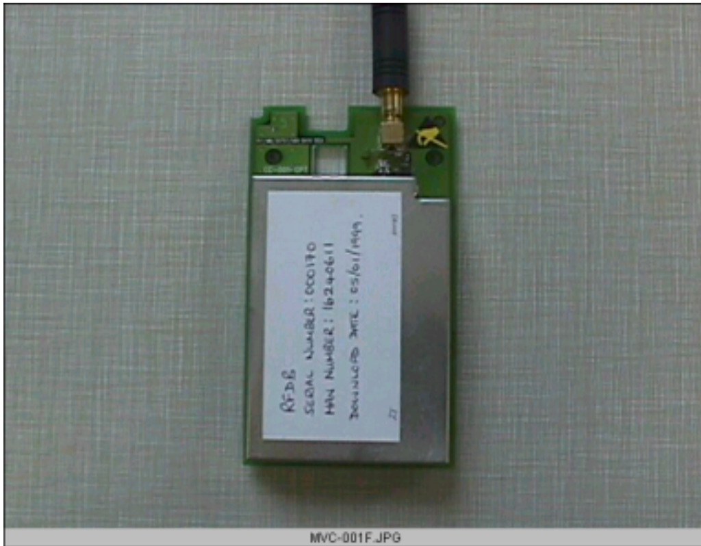
GPT Modem - Close Up of RF PCB Shielded Side
