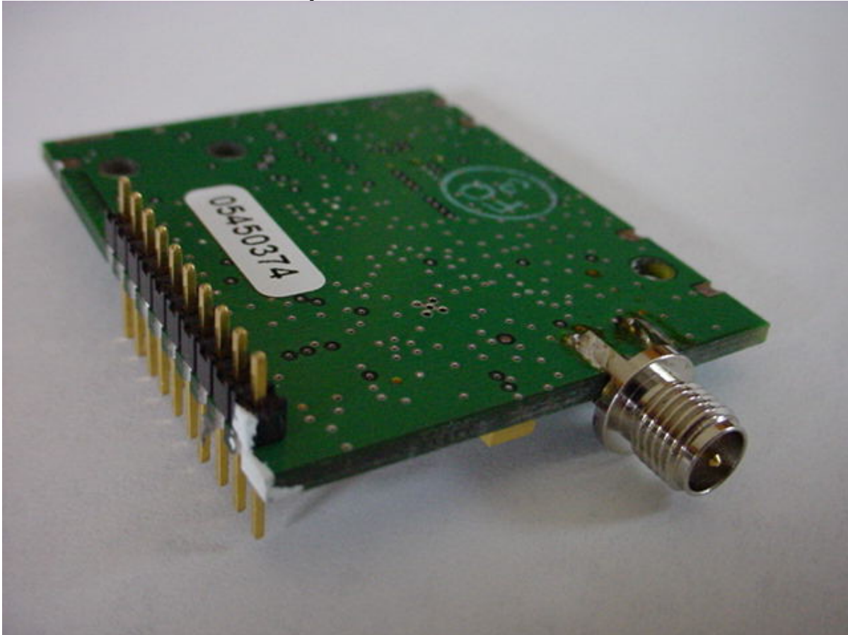
Photo Seven – External Close Up of Antenna Connector
