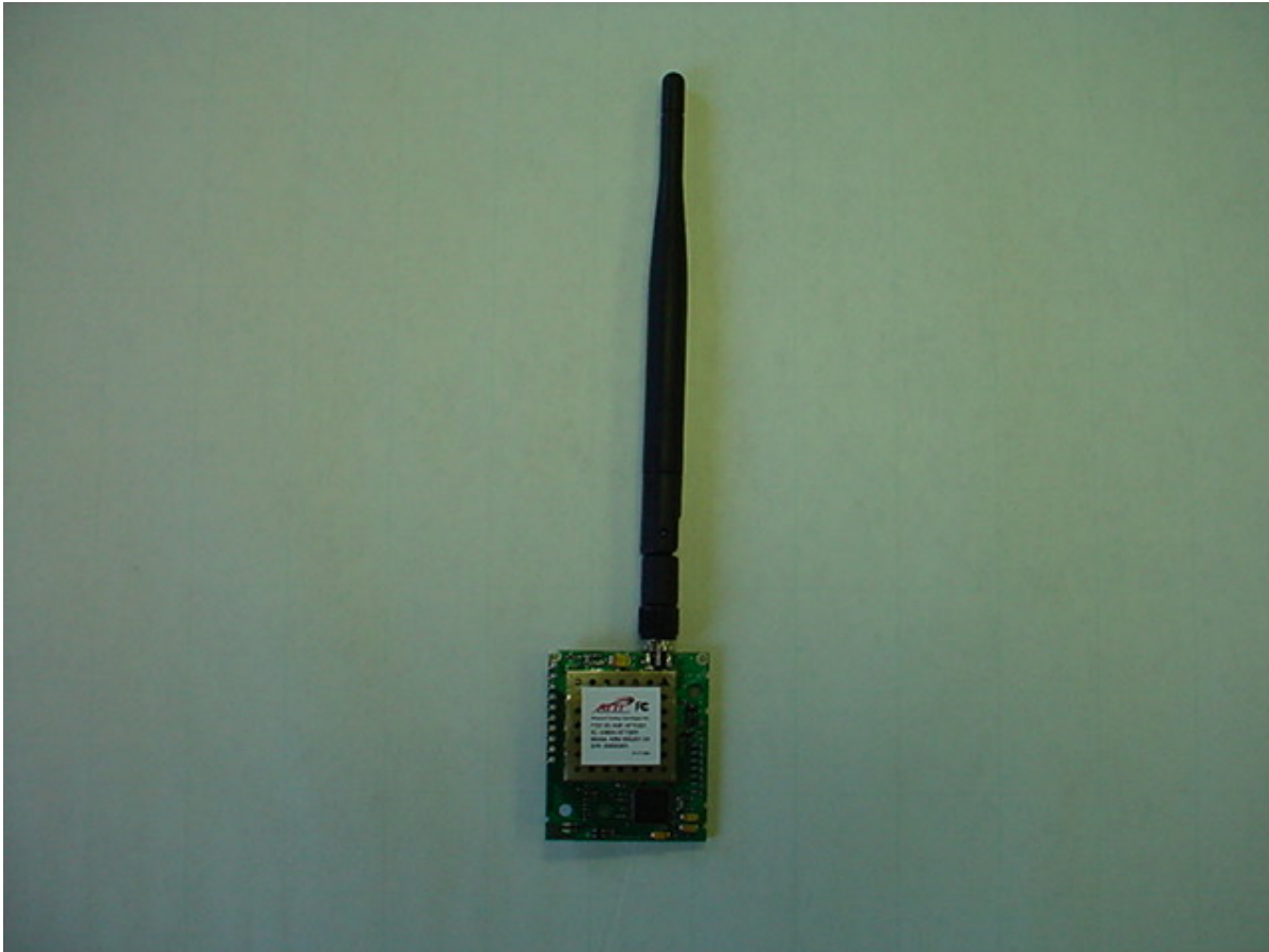
Photo Five – External RF Section with Antenna Connected
