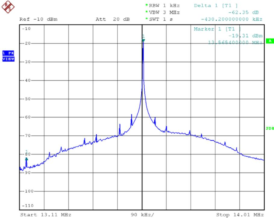
Bandedge Plot – Pursuant to FCC Part 15 Section 15. 225 Requirement      (Pass)
