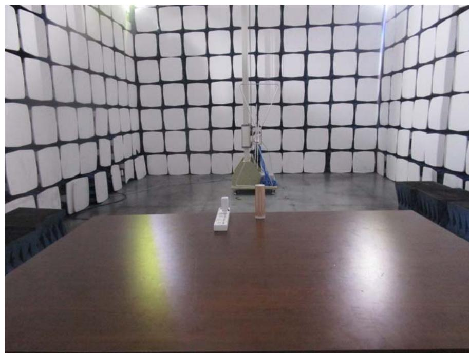
**Radiation Emission Test Setup (Above 1GHz)**
