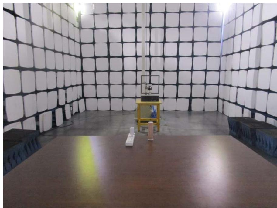
**Radiation Emission Test Setup (30MHz to 1GHz)**
