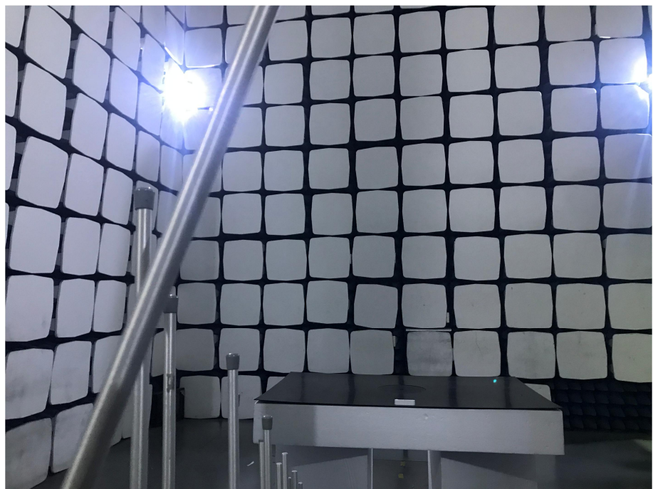
Radiation Emission Test Setup (30MHz to 1GHz)
