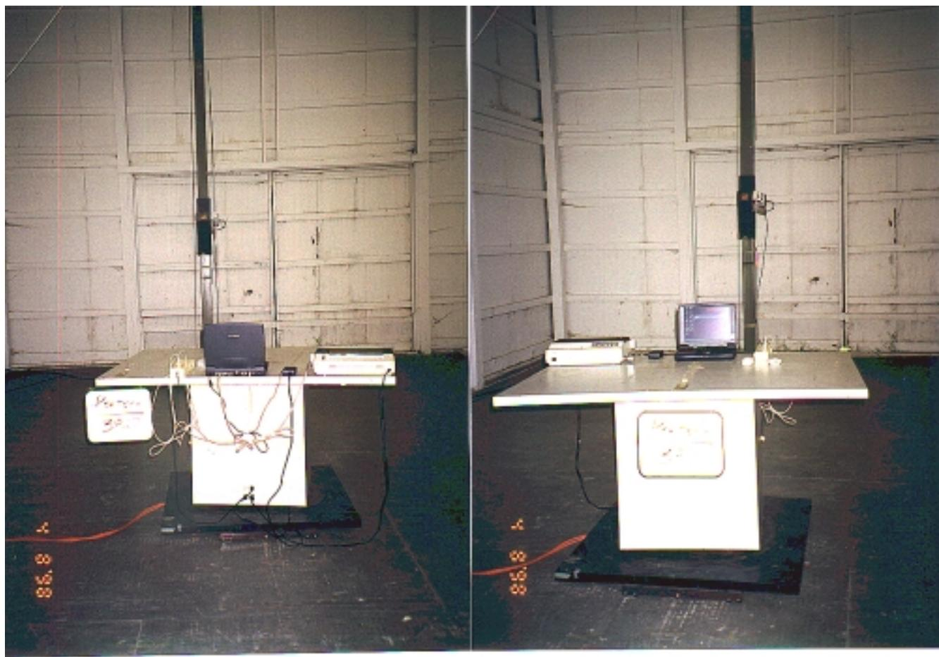
Test Setup Photos of Conducted Emissions
