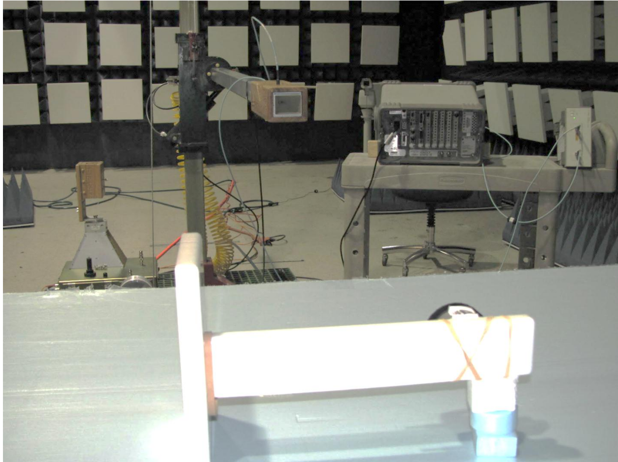
Figure 3: Radiated Emissions at 1m – 18 GHz to 26.5 GHz.
