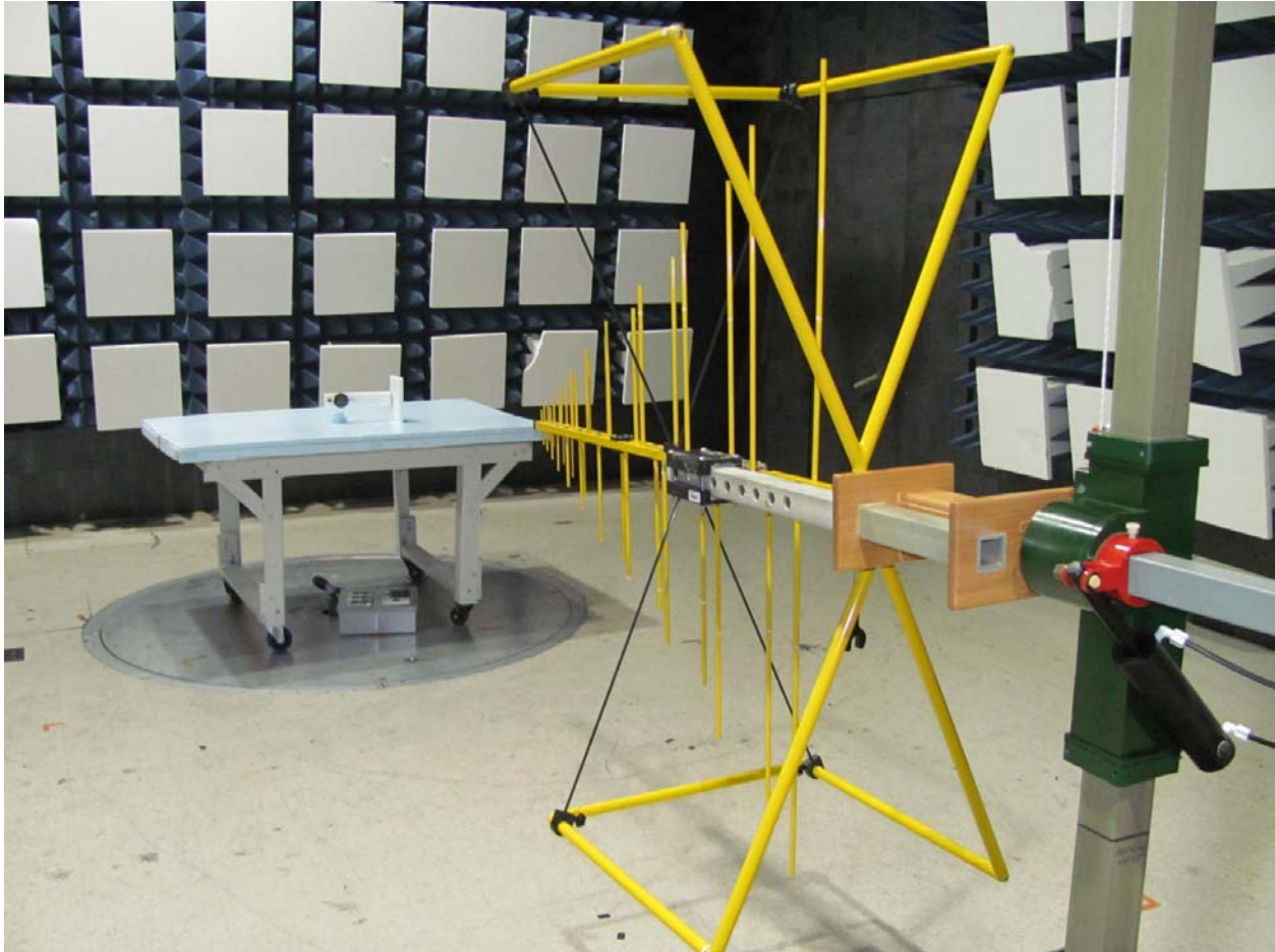
Figure 1: Radiated Emissions – 30 MHz to 1000 MHz.
