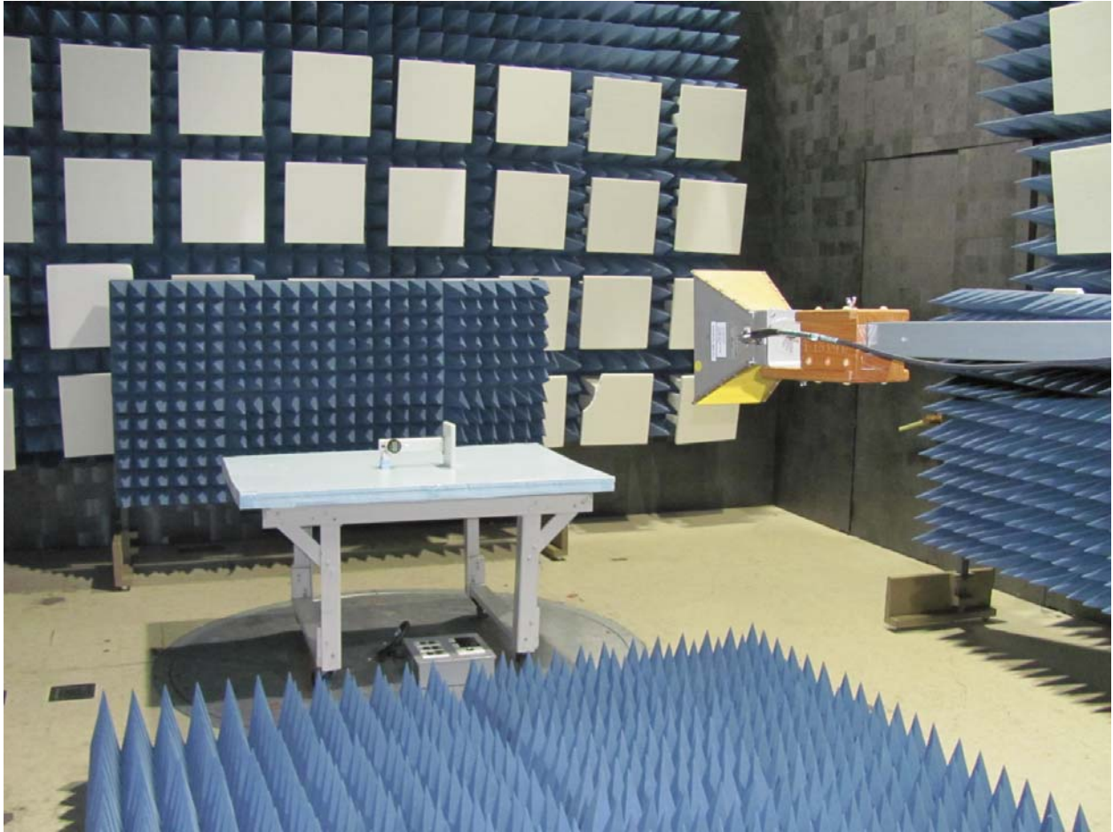
Figure 2: Radiated Emissions at 3m – 1 GHz to 18 GHz.
