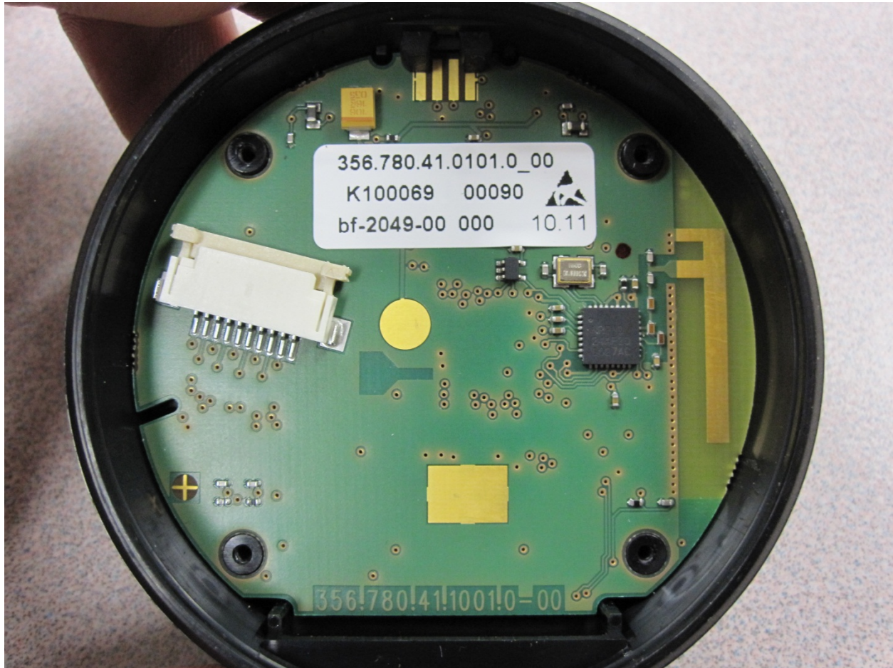
Figure 1: View of circuit board with transmitter inside the case (behind the digital display).
