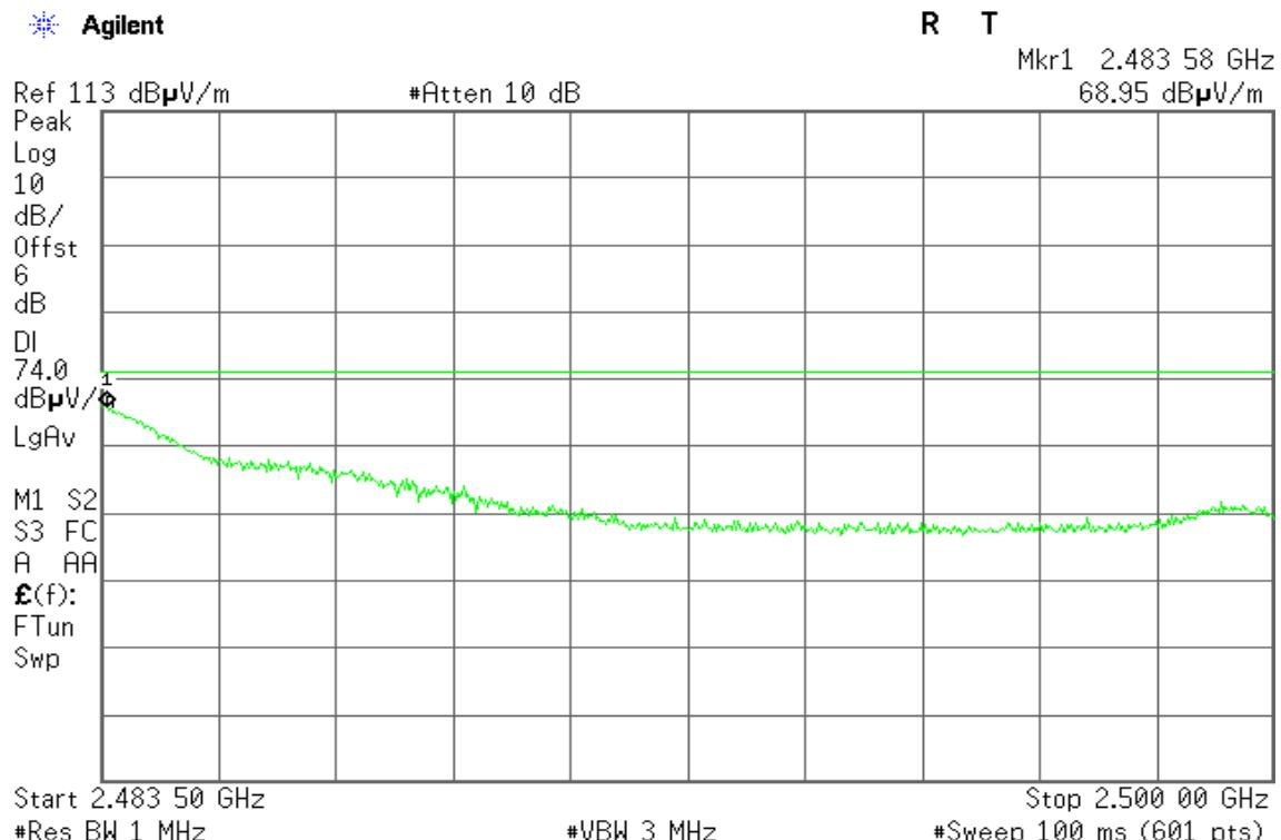
**Detector mode: Average****Polarity: Vertical**
