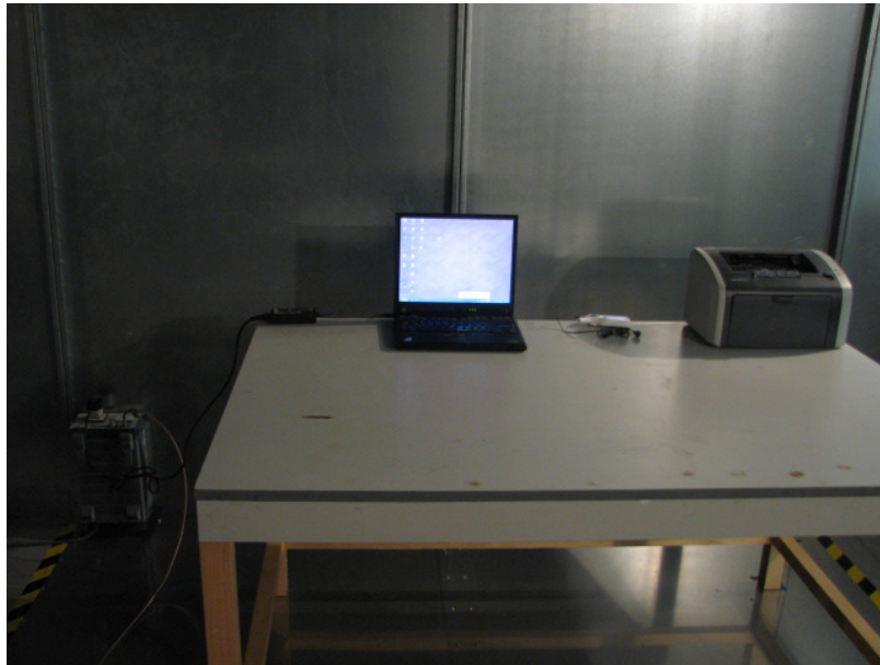
Set-up for Disturbance Voltage on AC Mains
