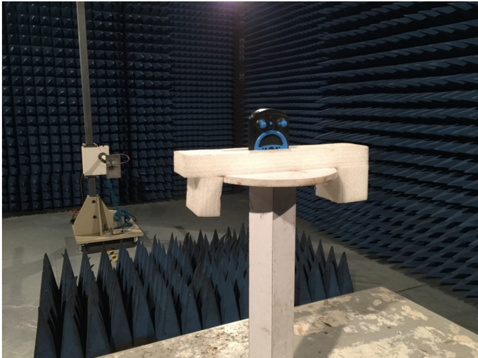
Setup for radiated emission
