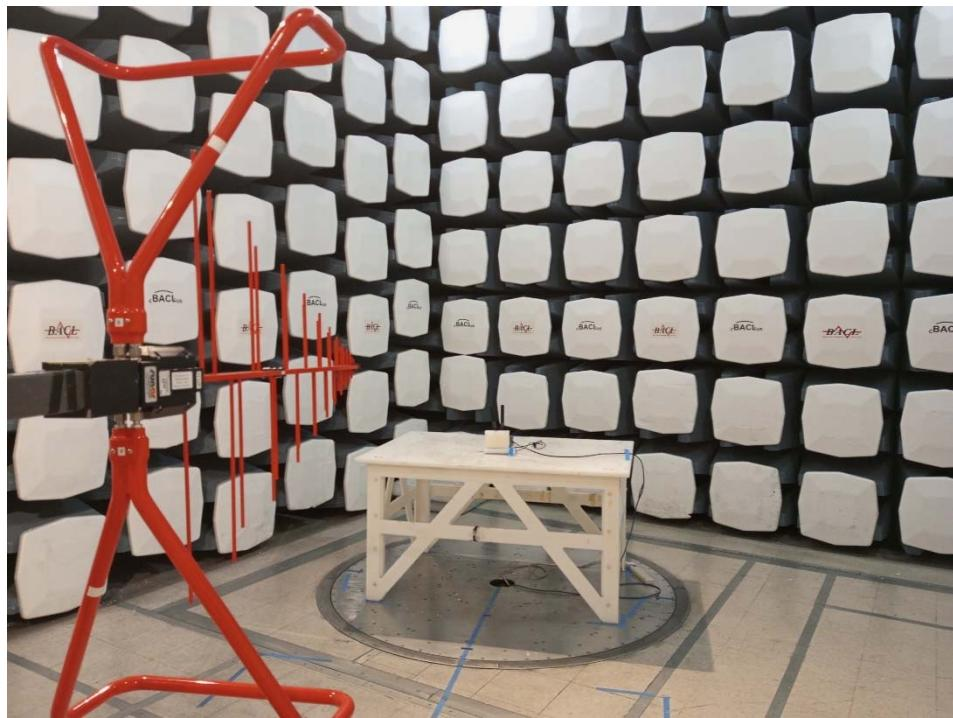
**1.6 Radiated Spurious Emissions: 30 MHz to 1000 MHz, Rear View at 3 meters distance**
