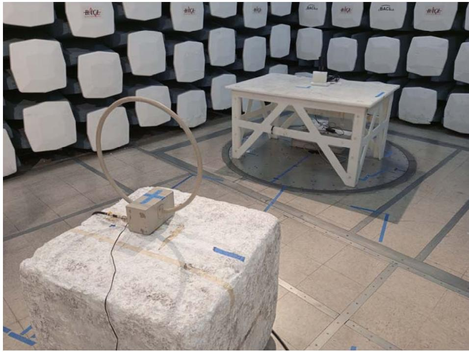
**1.4 Radiated Spurious Emissions: 9 kHz to 30 MHz, Parallel, Rear View at 3 meters distance**
