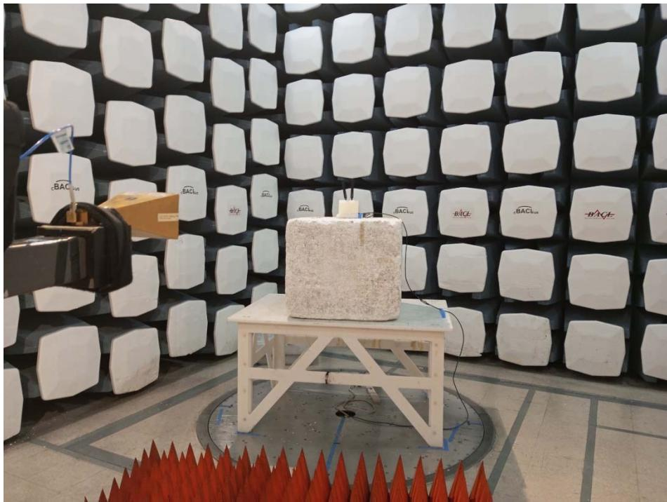
**1.10 Radiated Spurious Emissions: 18 GHz to 26.5 GHz, Rear View at 3 meters distance**
