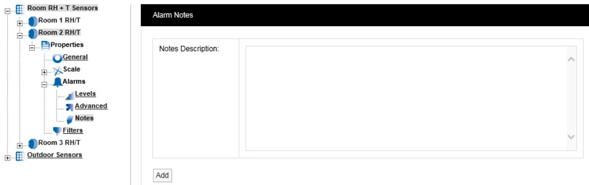
This feature allows you to enter notes for an Alarm. This is especially useful for inexperienced operators. The system can be set up so that low-level users can monitor the system but can't make changes. The Alarm Notes will give an inexperienced user specific instruction on what to do when an Alarm occurs.
