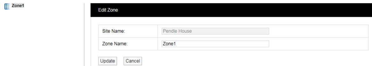
Select a name for the Zone that will make it easy to identify either the type of sensors in the Zone or the location of the Zone. In this example we are changing the Zone1 name to 'Room RH + T Sensors'. Enter the name into the **Zone Name** field, once happy select **Update**, see below.
