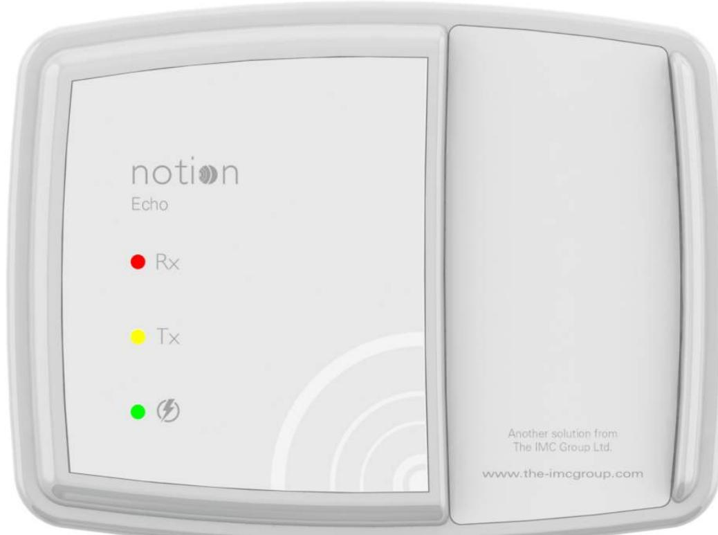
The Echo module provides a Repeater function for transmitted signals, should this be required in your installation. Key features:
