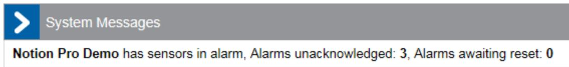
The **System Messages** inform you of where on the system the Alarms are. Once this window is closed the System Message bubble changes to amber which indicates that there are still live messages but there are no new ones since the last time the System Messages were checked, see example below.
