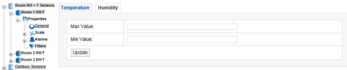
To activate this feature enter the required Min and Max values in the appropriate fields. The values should be whole numbers in the range 50 for the Max Value and -40 for the Min Value. Select Update when finished. (A warning message is given if you click on another tab before you've selected Update for a change you made on the current tab.) Once the data is accepted you will see the following screen, see below.
