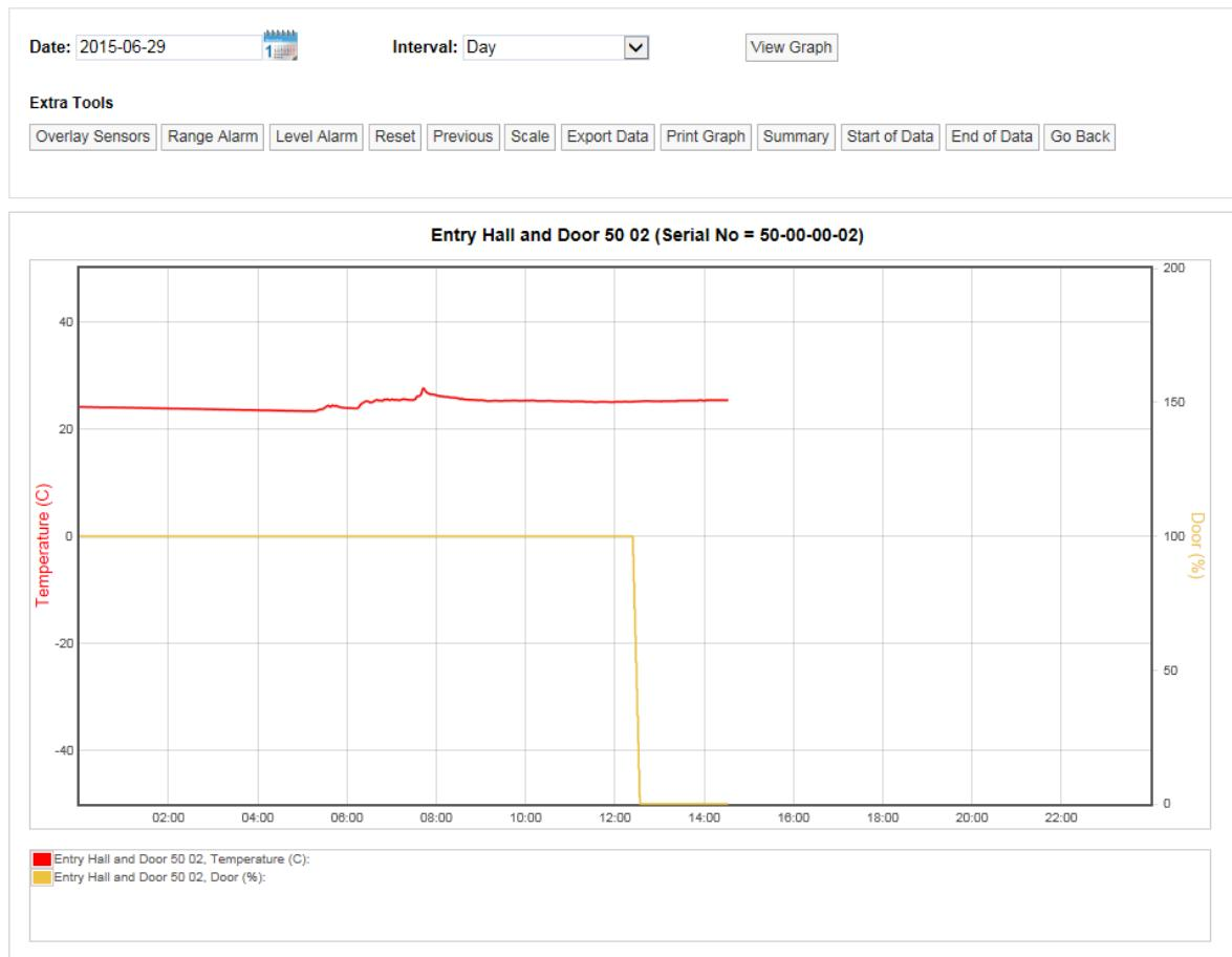
Here we see temperature data in red, door data in yellow. The door had been open (and so in an alarm state) until about 12:30, then somebody closed the door.
