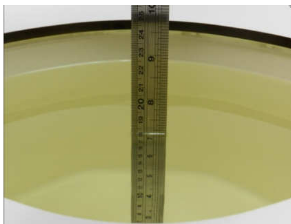
Fig 10.2 Photo of Liquid Height for Body SAR
