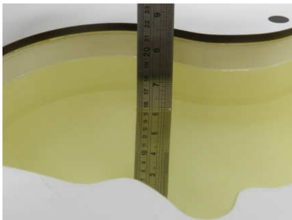
Fig 10.1 Photo of Liquid Height for Head SAR
