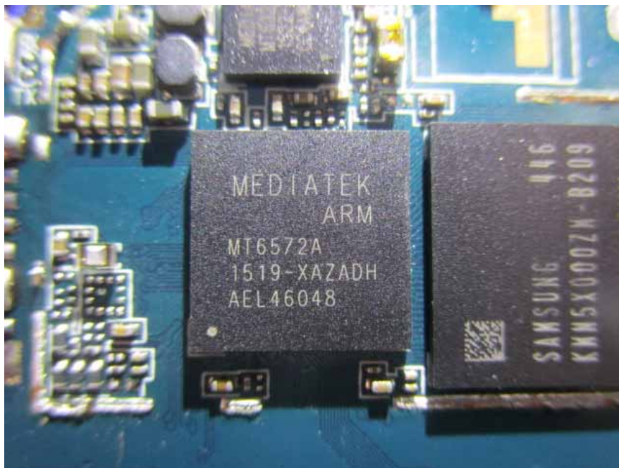
EUT –Main Chip View
