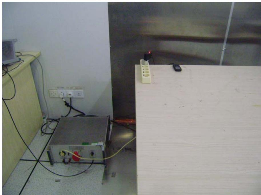
**Radiation Emission Test Setup (30MHz to 1GHz)**
