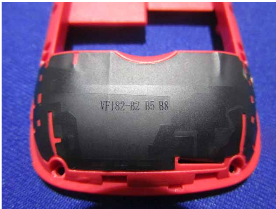
EUT –GSM/WCDMA Antenna View
