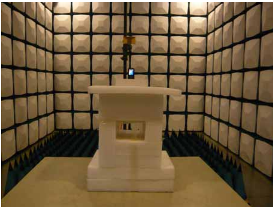
Radiated Emission View (Above 1GHz)
