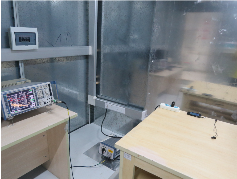
FCC LINE CONDUCTED EMISSION TEST SETUP
