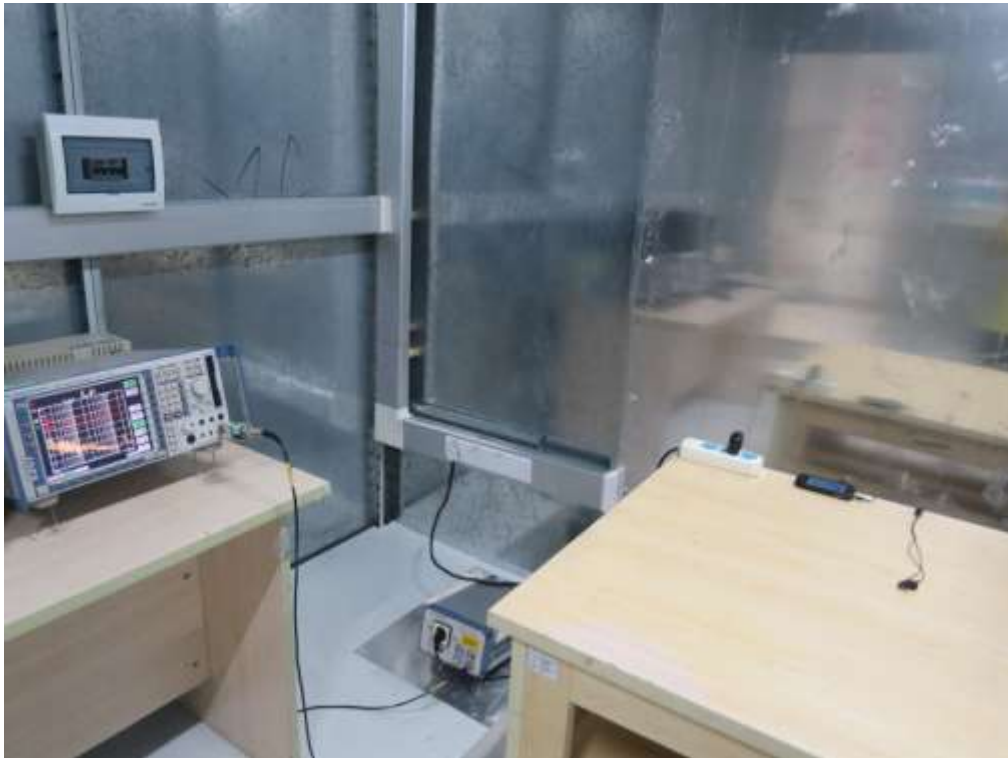
FCC RADIATED EMISSION TEST SETUP
