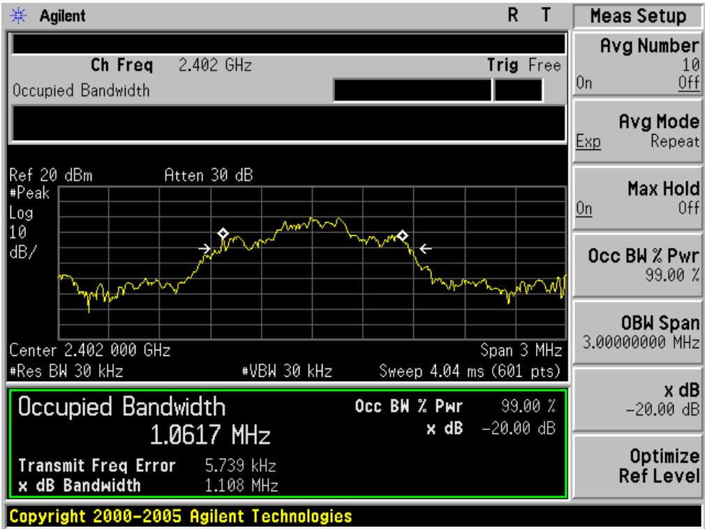
TEST PLOT OF BANDWIDTH FOR LOW CHANNEL
