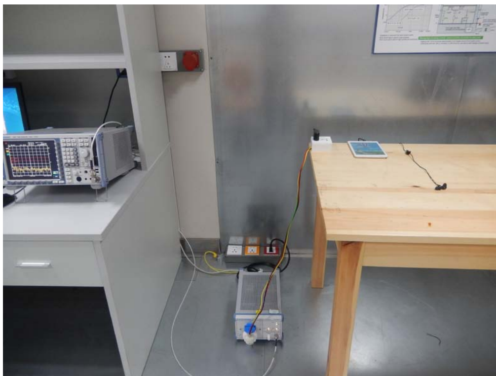
FCC RADIATED EMISSION TEST SETUP radiation L
